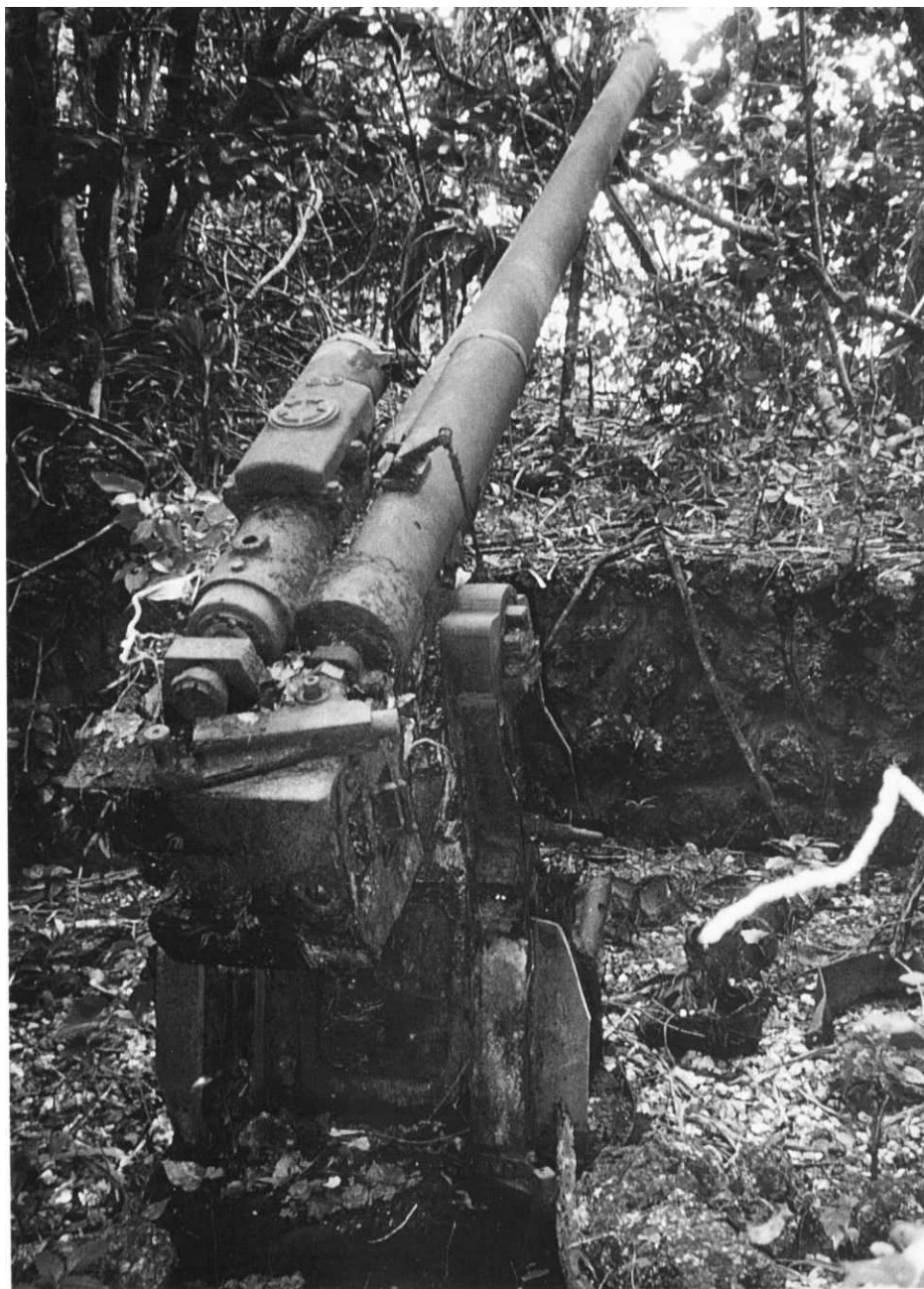
Caption and photo by Phillip D. Orr Possibly one of the best preserved specimens of its kind in the Pacific, this Model 10 120mm dual-purpose anti-aircraft and coastal defense gun is on the western shore of Ngesebus. The gun rests on its skid plate and was sited in a natural position.
