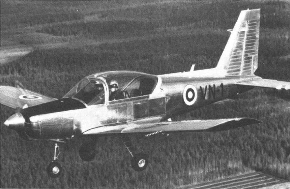
Finnish-built L-70 Vinka elementary trainer produced by Valmet Courtesy General Headquarters, Finnish Defense Forces
