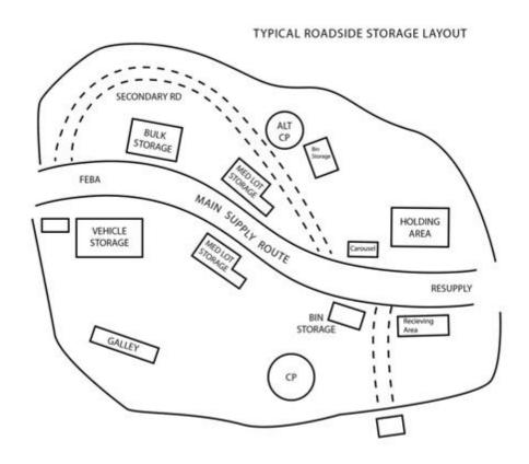
Figure 3-1. Typical Roadside Storage Layout
