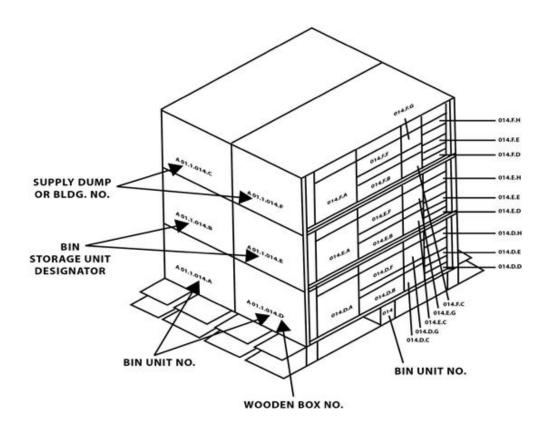
Figure M-8. Markings for Bin Storage Unit
