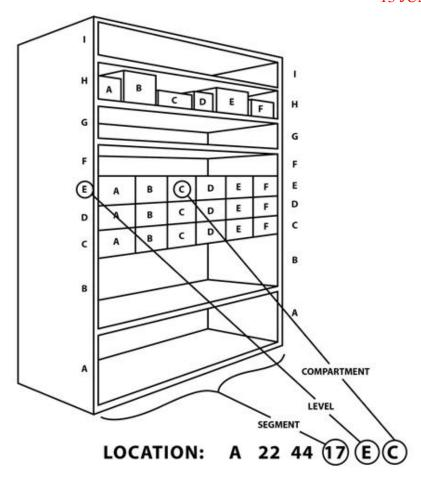
Figure M-5. Segment Level Compartment Bin Storage
