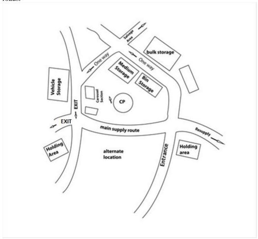
Figure 3-2. Typical Depth-Storage Dump
