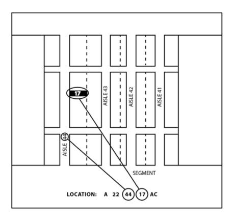
Figure M-3. Aisle and Segment Bulk Storage
