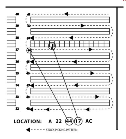
Figure M-4. Aisle and Segment Bin Storage
