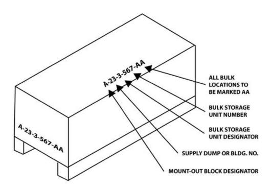
Figure N-1. Bulk Storage Units
