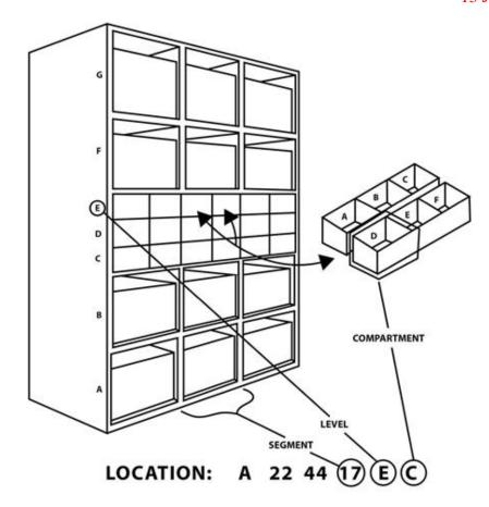
Figure M-6. Segment Level Compartment Divided Bin Storage
