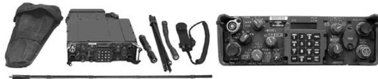
Figure 5-11. AN/PRC-119 (A-F), Single-Channel Ground and Airborne Radio System Man-pack Radio.
