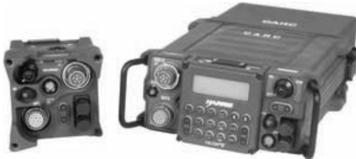
Figure 5-15. RF-5800R-RC111, Remote Control System.
