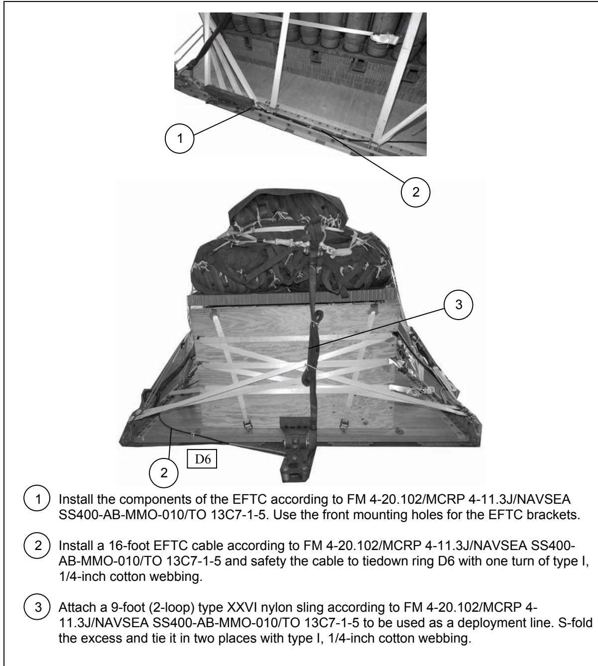
Figure 8-27. Extraction System Installed
