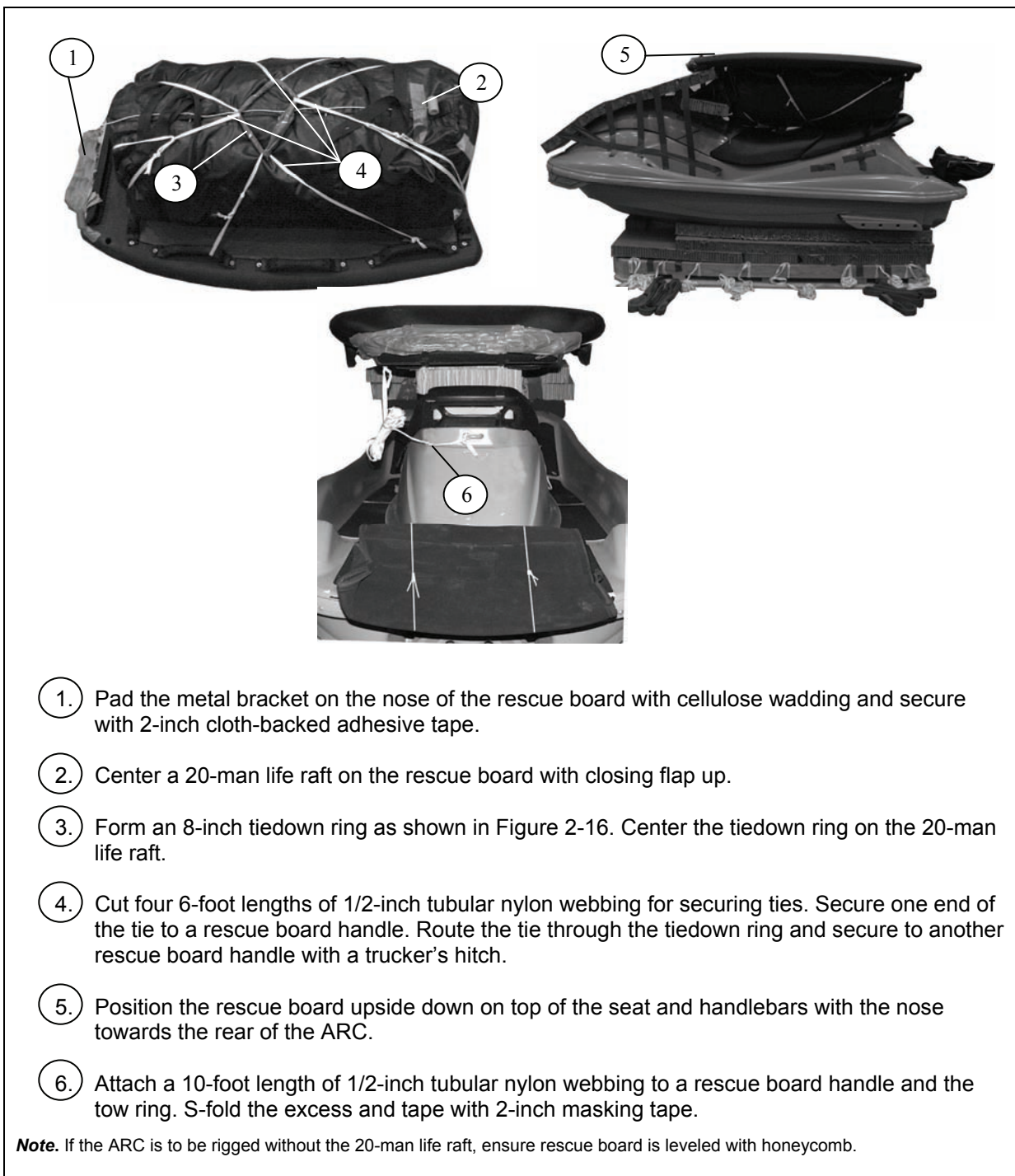
Figure 5-22. Rescue Board Installed
