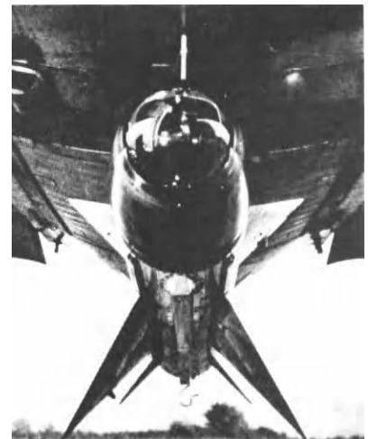
The Martel AJ168, pictured being carried by an RAF Buccaneer (also fitted with a video/command-link pod) and above, has a nose-mounted camera, whereas the AS37 has a pointed nose.
