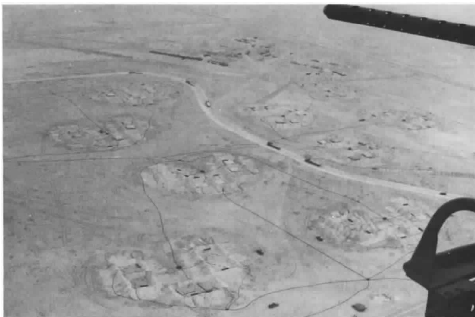
Part of the five-million-gallon bulk fuel farm in the southwest corner of the Direct Support Command's large combat service support base, 165 kilometers by dirt road west northwest of Al Mishab, photographed on 21 February 1991. The DSC built the vast base in seven days and it was enclosed by 42 kilometers of blastwall berm, a portion of which can be seen near the top of the photograph. The remote area had no place name so the DSC dubbed it "Al Khanjar," Arabic for a type of short sword.
