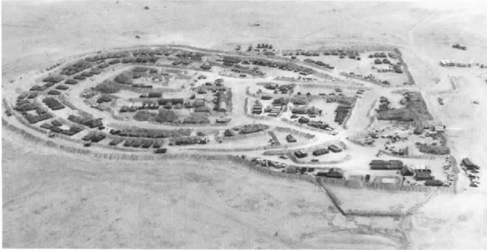
Aerial view photographed looking east on 21 February 1991, of the I MEF main command post located about eight kilometers south of the Al Khanjar Combat Service Support Base. Concentric design of blastwall berms was for ease of defense by the command element's small security force. The site was located within a slight undulation of the terrain and could not be seen on foot beyond about two kilometers. The CP's radio antennas were removed away from the site.
