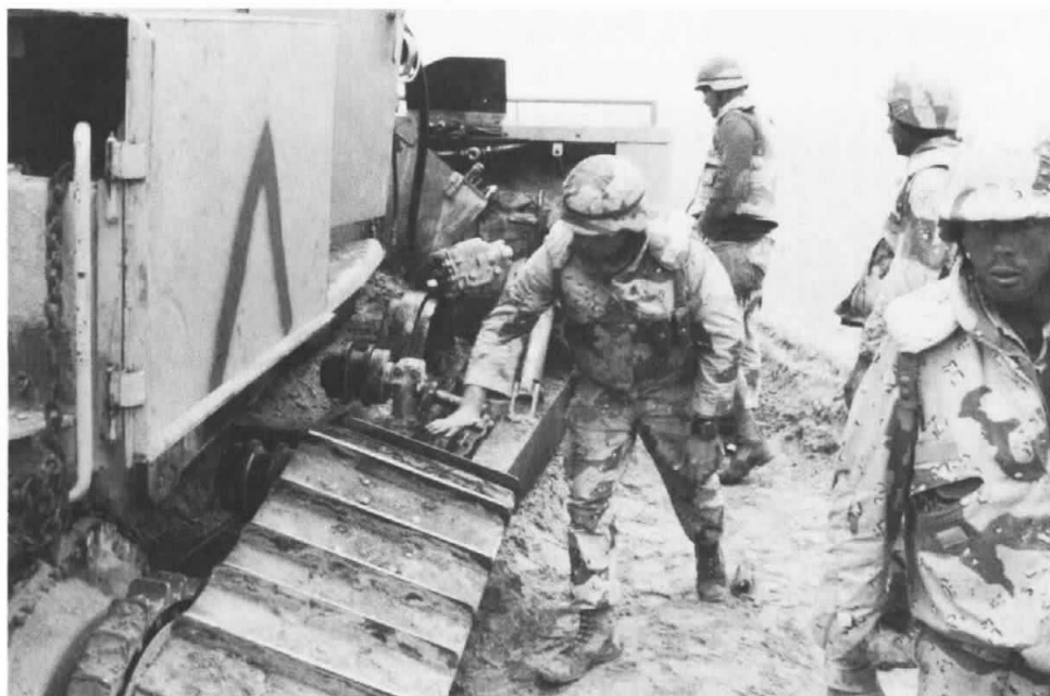
A Direct Support Command armored D-7 Caterpillar was disabled by a mine while attempting to widen Lane Blue 3 of the 2d Marine Division's breach. The division's greatest equipment losses occurred during the breaching operation and included seven M60 and one M1A1 tanks equipped with track-width mine plows, plus three assault amphibious vehicles.
