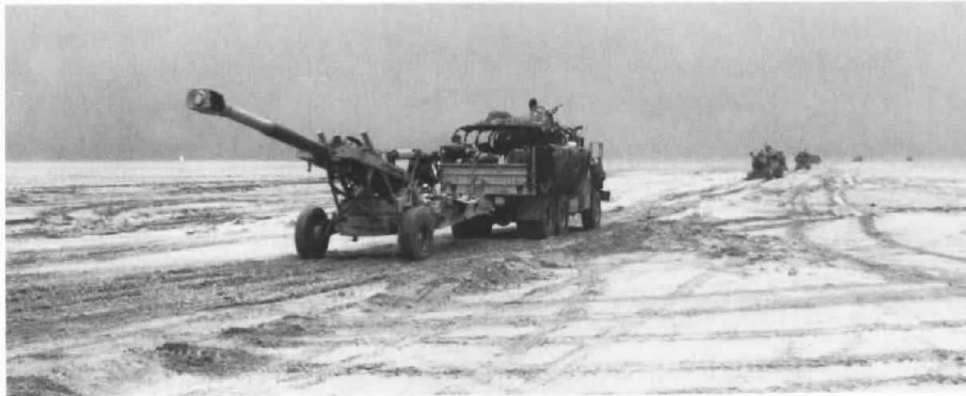
Trucks hauling artillerymen and M198 howitzers of the 5th Marine Expeditionary Brigade, 1 MEF's reserve force, negotiate the half-meter-deep mud of a sabkha (salt flat) near the 2d Marine Division's outer breaches on the morning of 27 February 1991. They are near the end of an all-night road march from blocking positions south of Al Wafrah. Iraqi combat engineers located their minefield barrier just inside areas of sabkha's to further obstruct attackers, but in general, trafficability on the battlefield was good.
