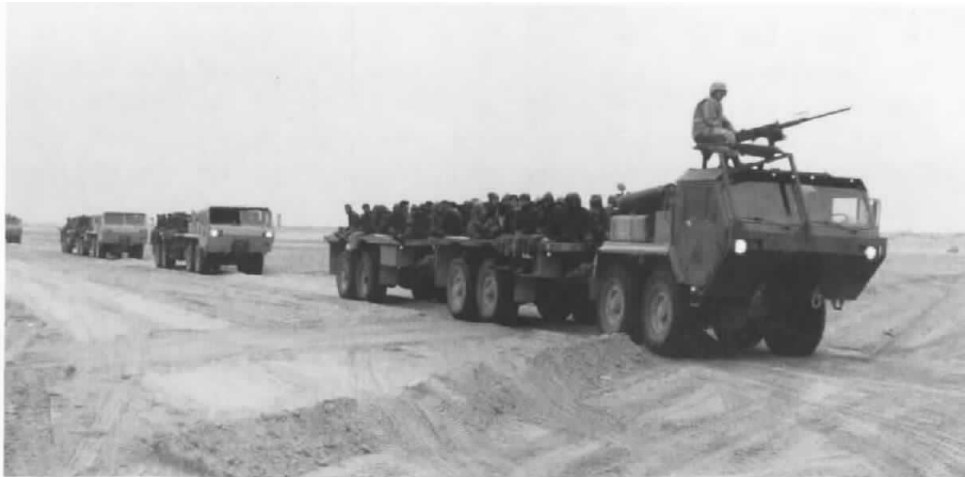
Iraqi prisoners-of-war being transported to holding facilities in Saudi Arabia on returning logistical vehicle systems (LVSs) of the Direct Support Command's 8th Motor Transport Battalion. The workhorse LVSs logged over one million miles and turned in a remarkable 93 percent serviceability rate.
