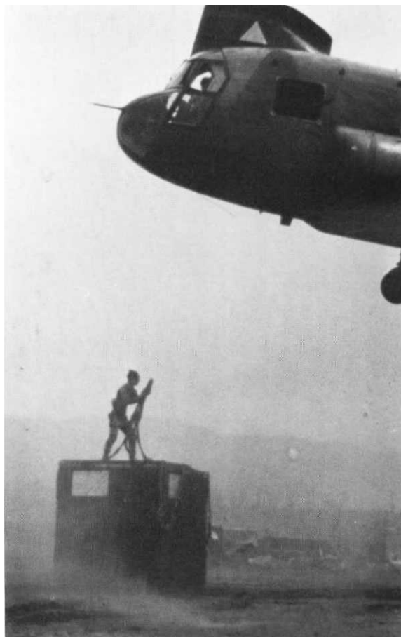
Courtesy of Col John G. Miller, USMC (Ret) A U.S. Army Boeing Vertol CH-47 resupply helicopter hovers at Khe Sanh, while a U.S. Marine advisor is about to hook up the container to the aircraft.
