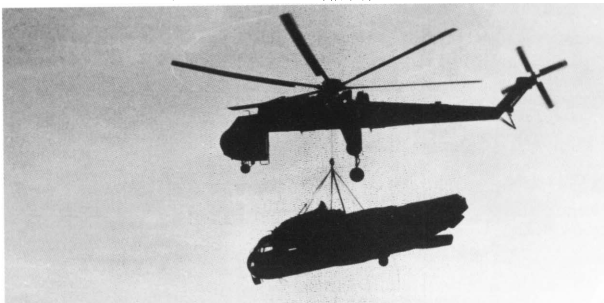
Top photo is from the Abel Collection and bottom photo is courtesy of Col Roger W. Peard, USMC (Ret) Top, a Marine Sikorsky CH-53 Sea Stallion lifts a damaged Marine Sikorsky UH-34D Sea Horse from the landing strip at An Hoa. Below, a crashed CH-53 Sea Stallion, itself, is lifted by an Army Tarhe CH-54 Sky Crane back to MAG-16 at Marble Mountain. The Army helicopter could lift up to 20,000 pounds.
