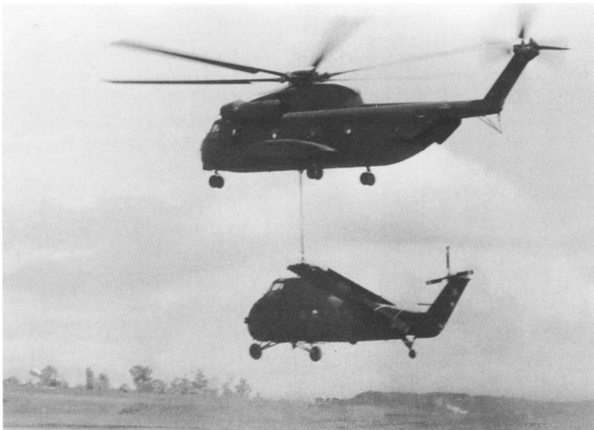
Top photo is from the Abel Collection and bottom photo is courtesy of Col Roger W. Peard, USMC (Ret) Top, a Marine Sikorsky CH-53 Sea Stallion lifts a damaged Marine Sikorsky UH-34D Sea Horse from the landing strip at An Hoa. Below, a crashed CH-53 Sea Stallion, itself, is lifted by an Army Tarhe CH-54 Sky Crane back to MAG-16 at Marble Mountain. The Army helicopter could lift up to 20,000 pounds.
