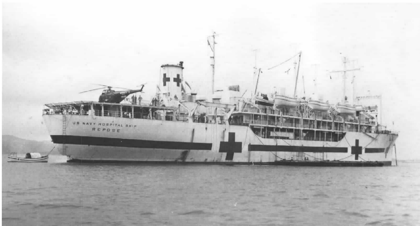
The hospital ship Repose (AH 17) at anchor in Incheon Harbor. Note the helicopter landing pad mounted on the ship's stern; this configuration became standard on all hospital ships during the course of the Korean War.
