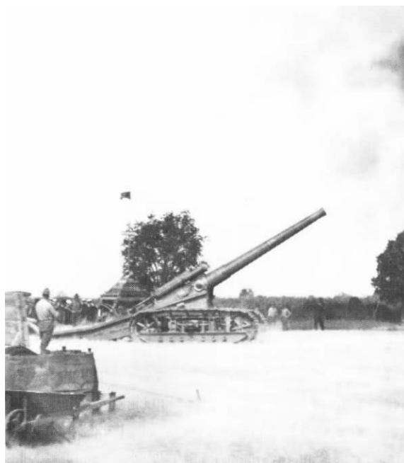
US Navy Photo PHD-6209 Marine and Navy gunners test-fire a 7-inch track-mount naval gun at Indian Head Naval Proving Ground, Maryland. During testing in October and November 1918, the gun crews fired the weapons up to 40 degrees elevation.
