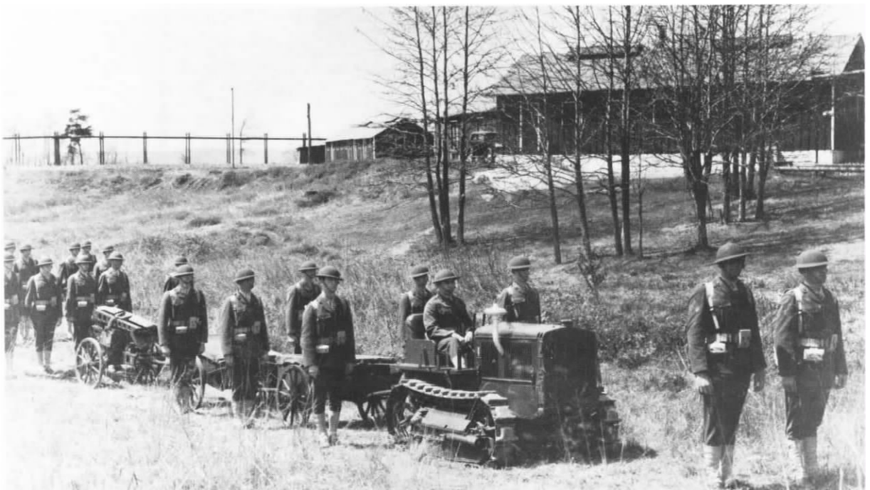
The 75mm pack howitzer battery shown in the previous picture is prepared to move out. Note that the trail of the gun has been removed and strapped to the barrel for transit.
