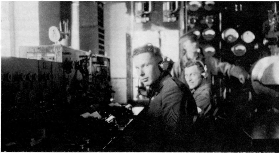
Fellow Marines man the "reception apparatus" at the American Legation's Station NPP, copying down Morse signals onto typewriters as they listen with earphones. The station's 2,500-watt long-wave transmitter could reach as far as Guam and Cavite.
