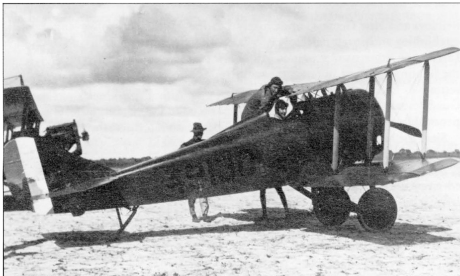
A "Tommy Morse Scout" powered by an 80-horsepower LeRhône engine, was photographed at Marine Flying Field, Miami, Florida, in 1915. Because of the Tommy's success as a trainer, it became one of the most popular single-seaters built in America.
