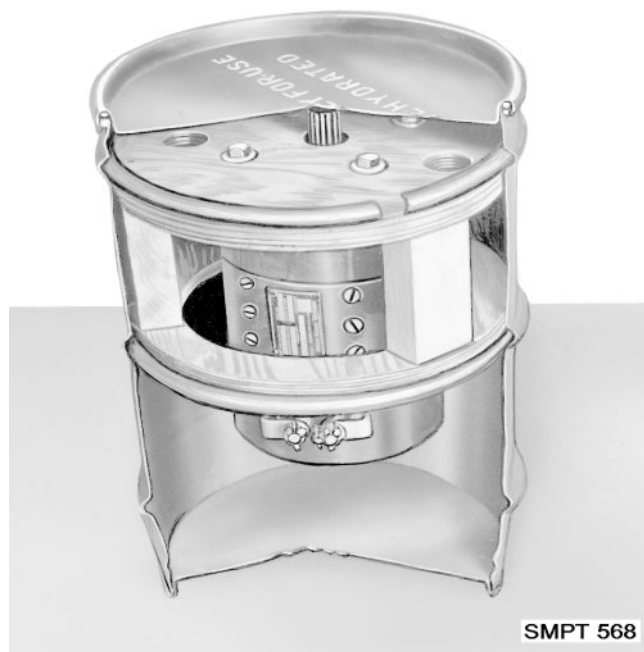
Figure 5-2. Internal locking rings in position (MIL-D-6054).
