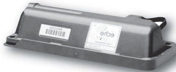
Figure 14-8. Active Radio Frequency Identification Tag.
