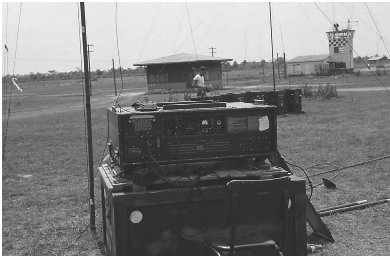
An AN/TRC-75 transmitter-receiver was set up outside of the communications center. The poles in the background supported the long-wire antennas that attached to the radio.
