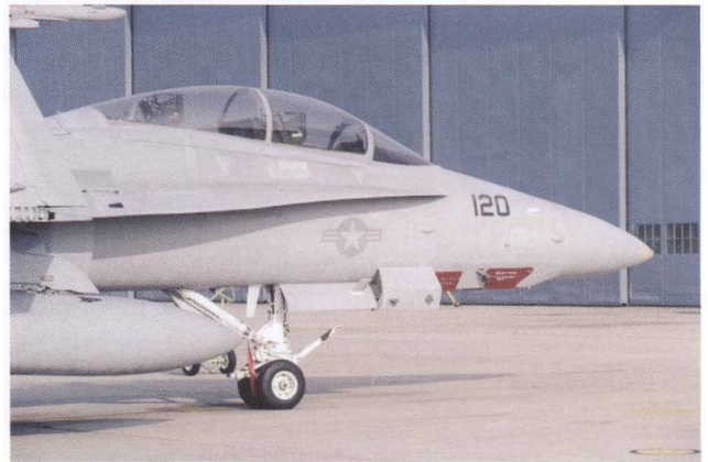
A 3 d MAF F/A-18D with an ATARS imagery pod installed. This aircraft provided imagery in support of the MEF's targeting effort.
