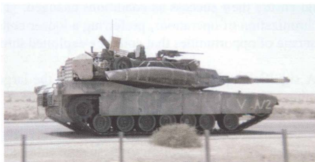
To extend the Division's logistical culminating point, vehicles were fitted with external fuel reserves, such as these FLEXCELL fuel bladders on an M1A1.
