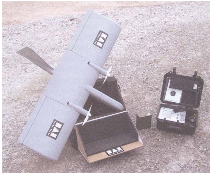
The manpackable Dragoneye UAV system would prove invaluable for decentralized intelligence collection at the Battalion level.
