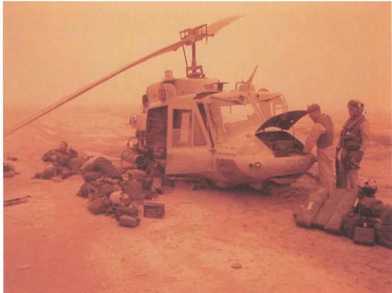
The sandstorm took its toll on machines as well as aircraft. This UH-1N crashed because of dirt and debris blown into the engine.
