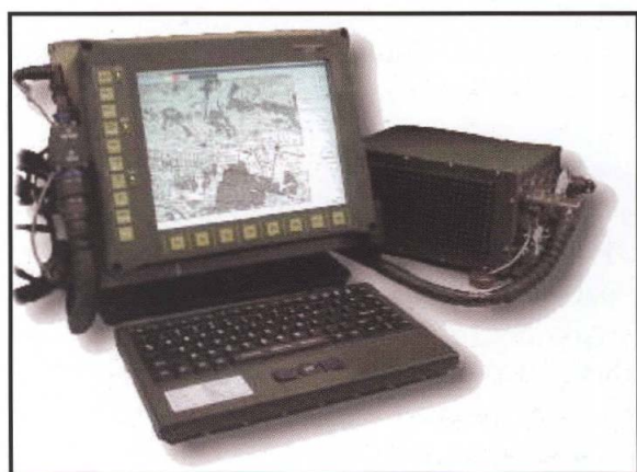
Mobile Digital Automated Computer Terminal. This equipment was installed in vehicles throughout the Division to provide immediate position reporting of friendly forces as well as rapid transmission of free-text messages.
