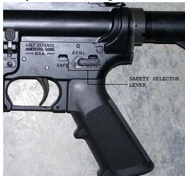
Figure 4. Selector Switch on Safe
