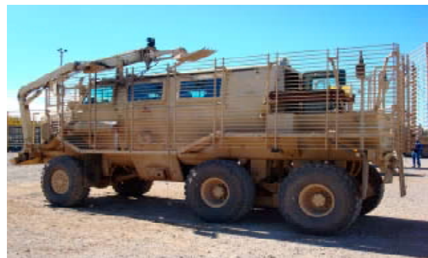
Buffalo, Route Clearance Vehicle has firsthand experience in what they are teaching the students."
