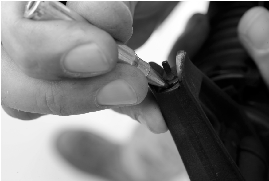
Figure 8-12. Front Sight Adjustment.
