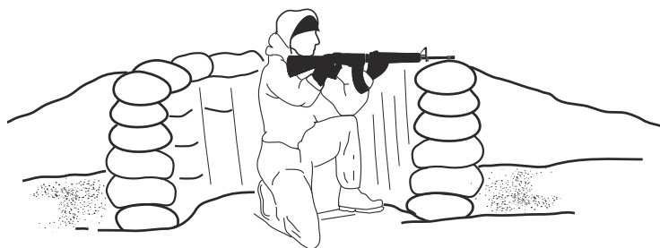
Figure 15-4. Fighting Position Using Sandbags.
