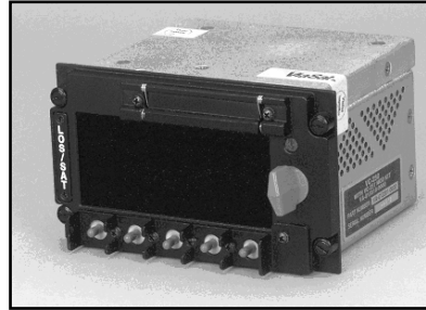
Figure F-1. Control/Fill Panel
