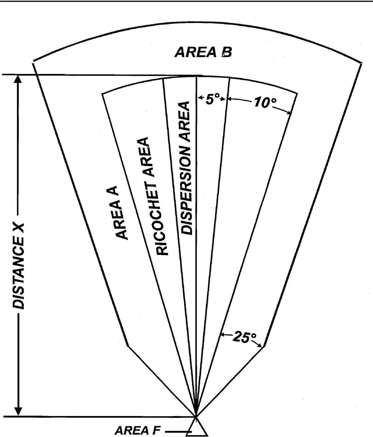
Figure 9-2. SDZ for firing recoilless rifles firing at quadrant elevation less than 15°
