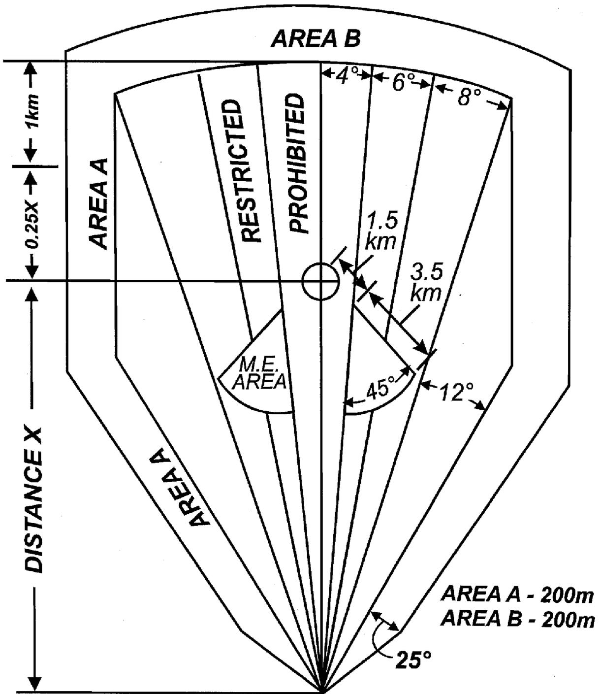
Figure 11-6. SDZ for firing Copperhead in the glide mode
