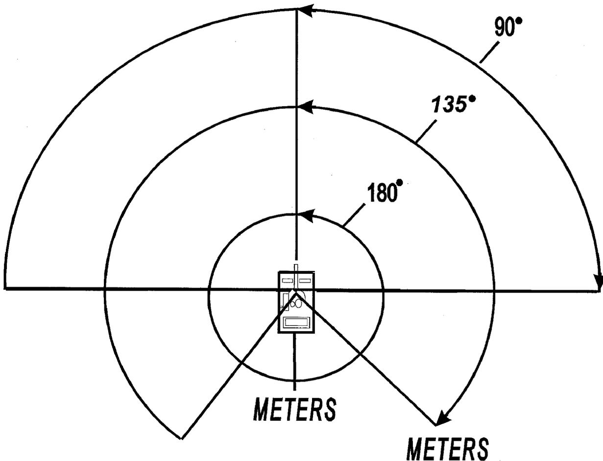
Figure 12-10. Hazardous impulse noise (140 dBP) contour zones
