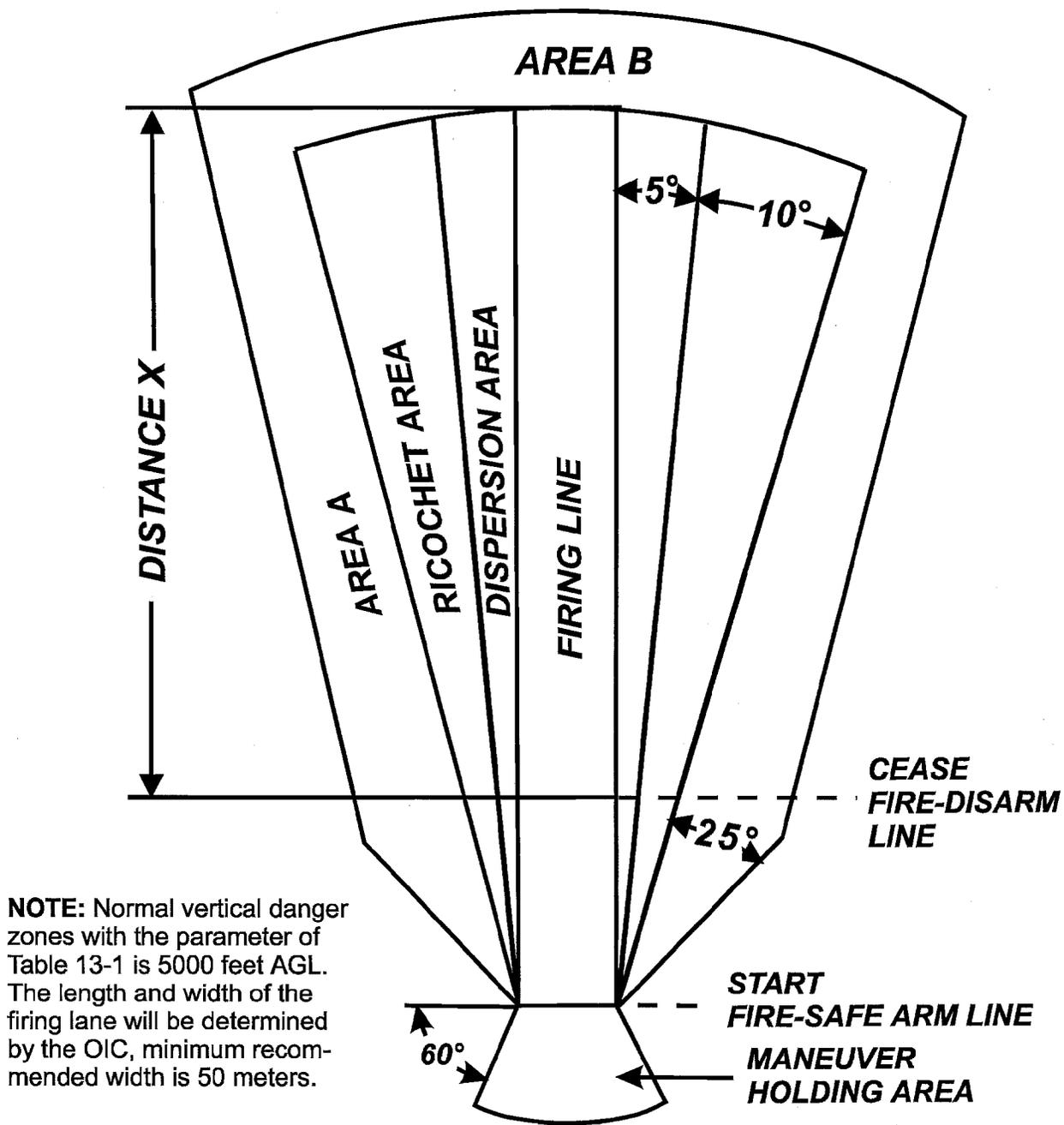
**NOTE:** Normal vertical danger zones with the parameter of Table 13-1 is 5000 feet AGL. The length and width of the firing lane will be determined by the OIC, minimum recommended width is 50 meters.
