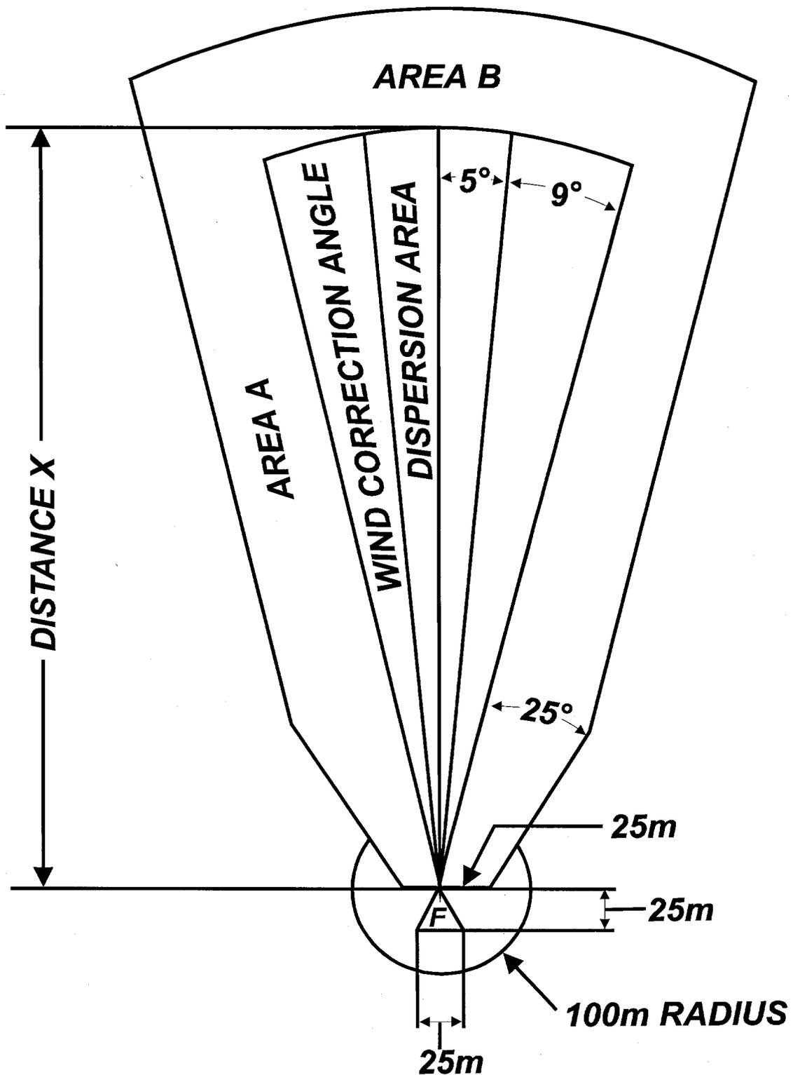
Figure 5-1. SDZ for firing ballistic aerial target systems
