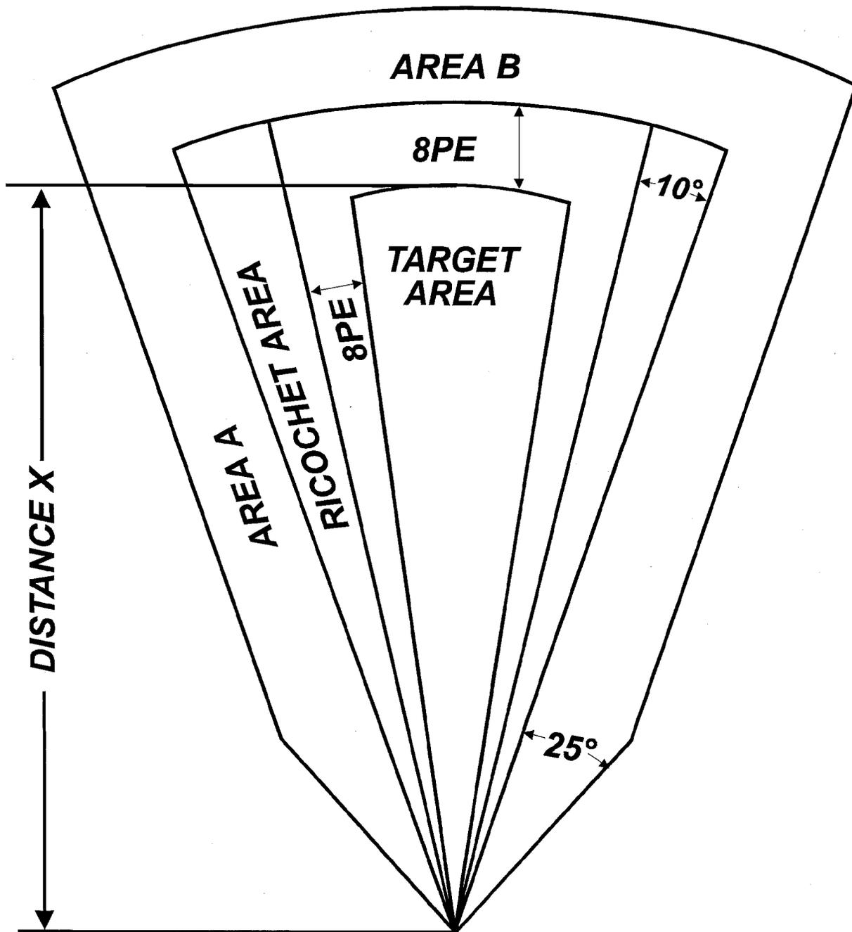
Figure 11-3. SDZ for firing field artillery cannon in the direct mode at fixed ground targets
