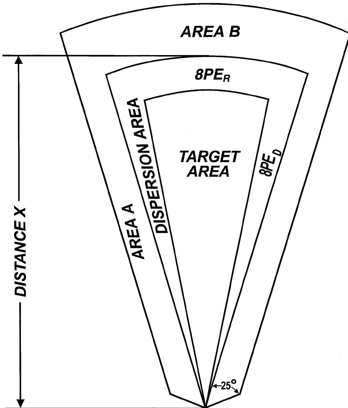
Note: The 25 degree angle must be increased to 70 degrees when firing HE ammunition at ranges equal to or less than 600 m for 60-mm mortars; 940 m for 81-mm mortars; 940 m for 4.2-in mortars; and 1,415 m for 120-mm mortars.
