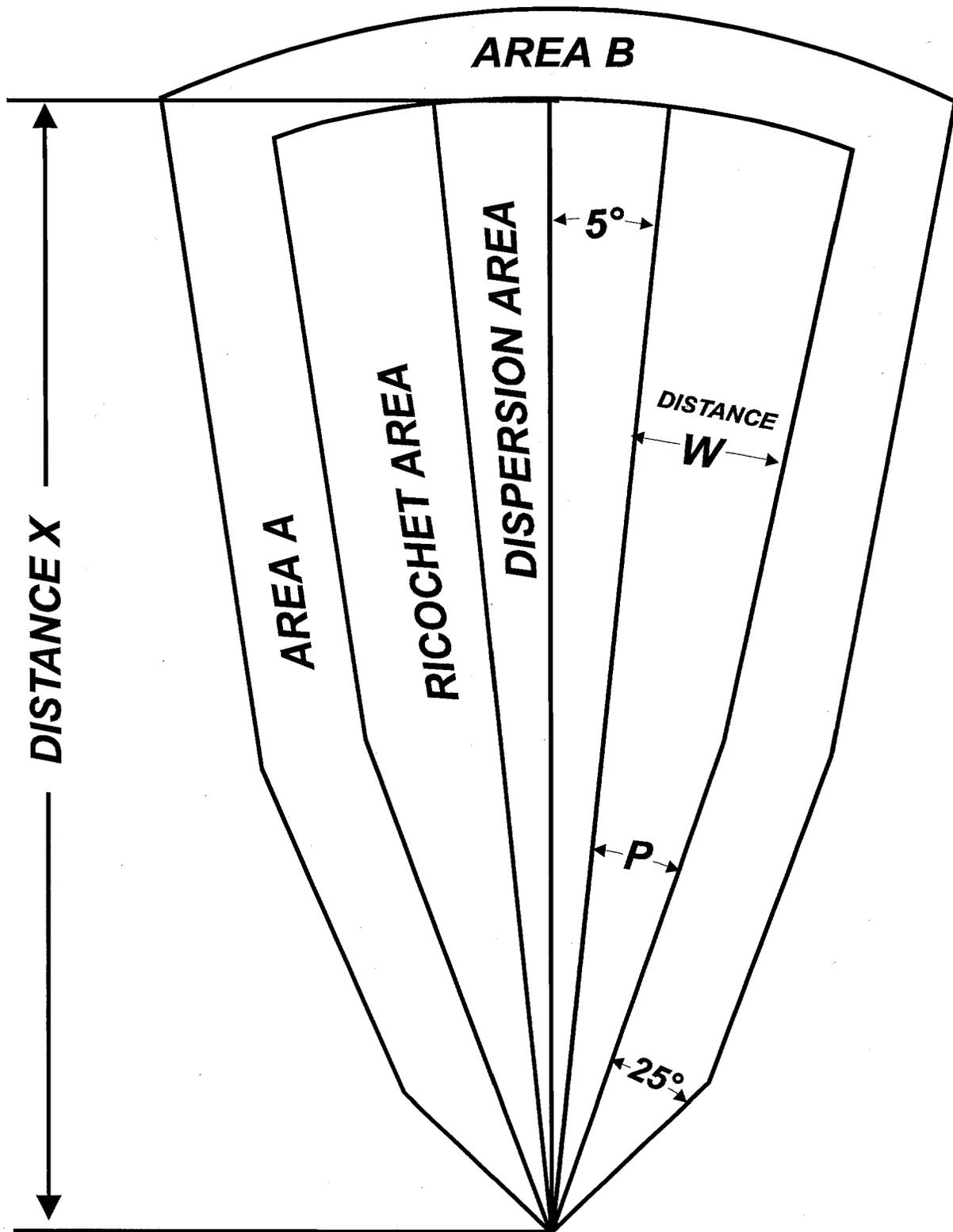
Figure 12-2. SDZ for firing select tank cannon cartridges
