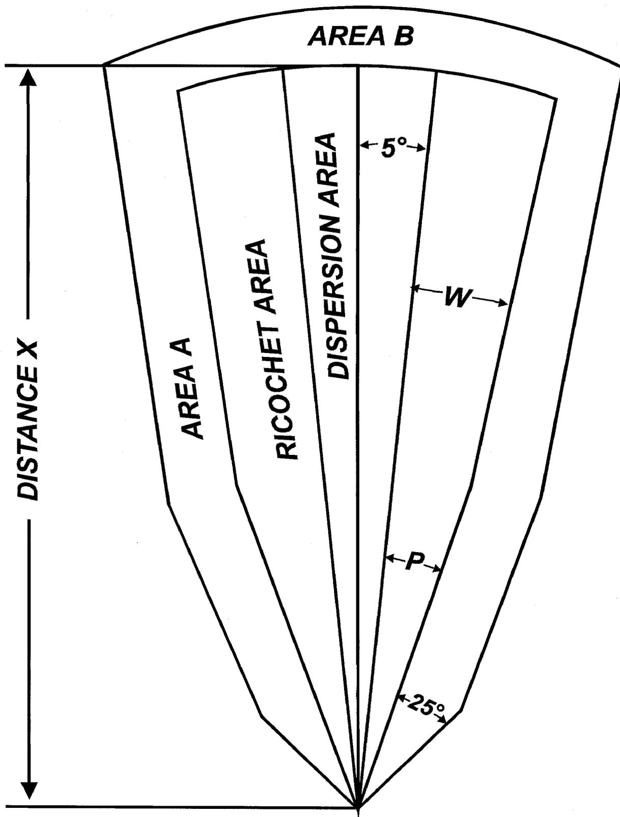
Figure 12-3. SDZ for firing 25-mm cannon cartridges
