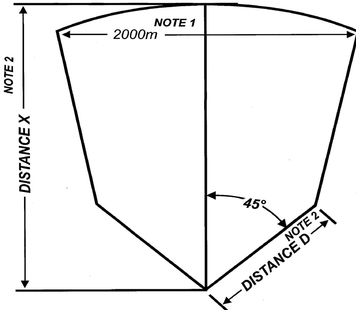
**WARNING:** Hardware discarded by the functioning of the projectile presents a potential hazard to unprotected personnel located to the side and rear of the weapon.
