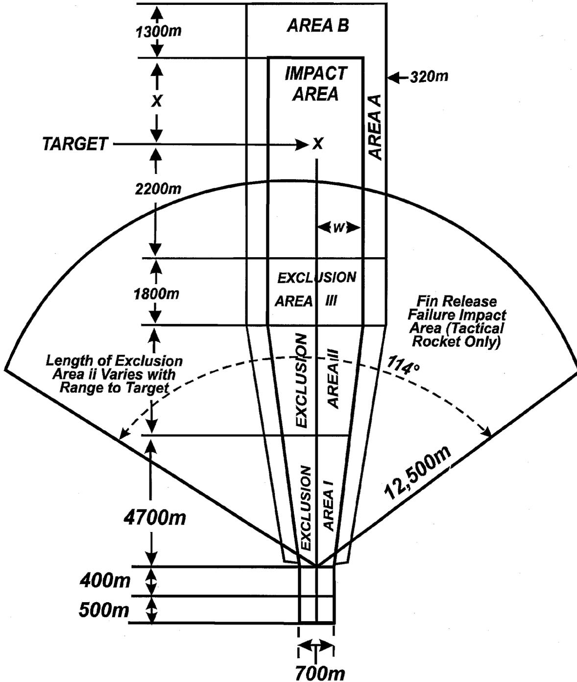
Figure 11-10. SDZ for firing multiple launch rocket system
