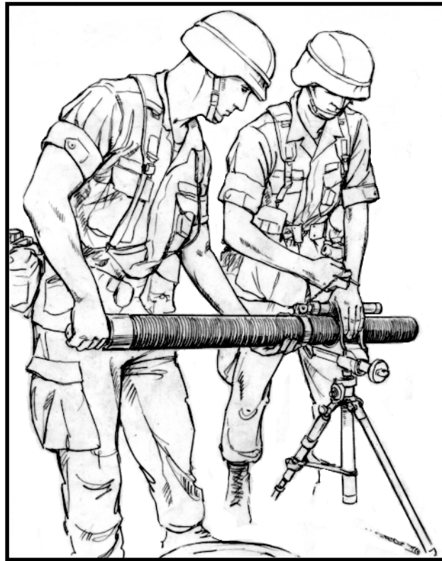
Figure 5-8. Bipod and mount attachment ring secured.
