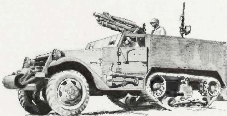
U.S. Halftrack Mounting a 75mm Pack Howitzer and a .50-Caliber Air-Cooled Machine Gun
