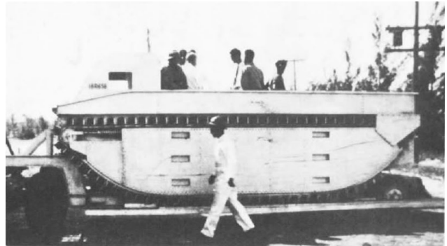
Roebling "Alligator 3" amphibian tractor is seen at Clearwater, Florida, in about 1940. The "Alligators" were developed, beginning in 1934, to cope with hurricane season flooding.
