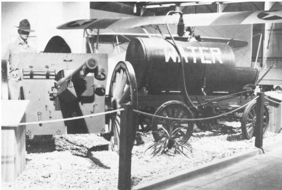
French 75mm gun M1897 is of the type which supported World War I Marines in France and continued in use by Corps artillery into the 1930s. The water wagon filled Marines' canteens and radiators during the Central American Banana Wars of the 1920s.
