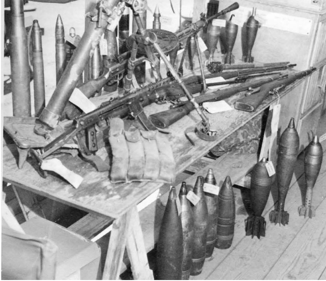
Deadly array of captured enemy weapons is displayed in the G-2 office tent at the 1st Marine Division's command post in Korea in August 1952. Included are a variety of mortar and artillery shells, machine guns, rifles, and a complete 60mm mortar.
