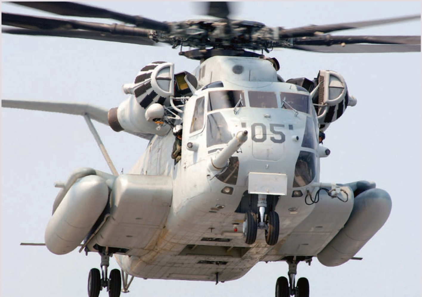
The refueling probe is the long mechanism sticking out of the lower front, right side of the helicopter. The Hercules aircraft refueled the Super Stallions three times during Operation Eastern Exit.
