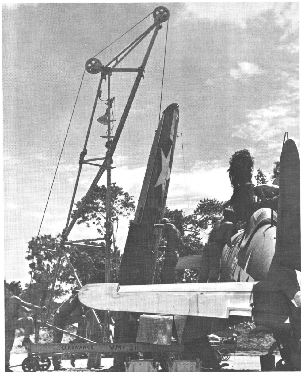
MECHANICS OF VMF-211 repair a Corsair which returned from a strike with its wings and fuselage full of holes from antiaircraft shell fragments. (USMC 77816)
