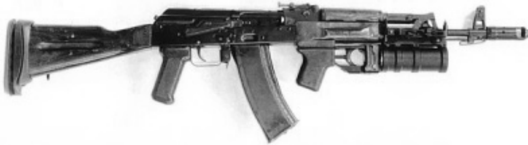
Figure H-11. BG-15 Grenade Launcher Mounted on AK-74.
