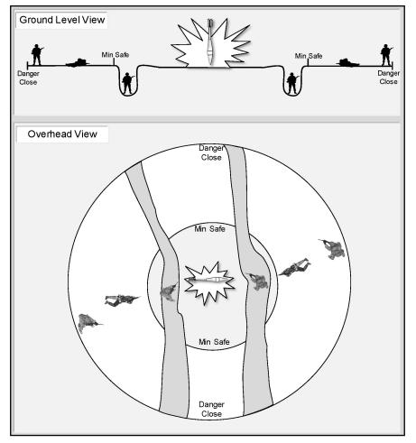
Figure 1-4. Example Minimum Safe Distance.
