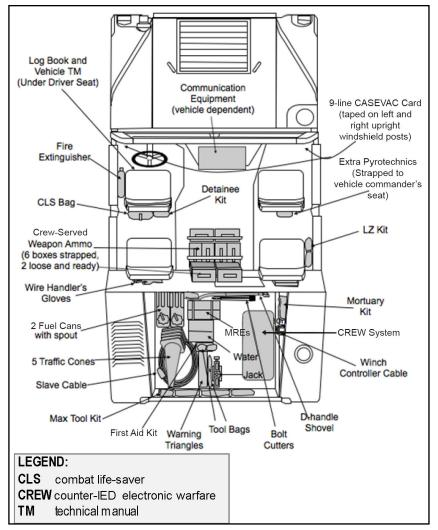
Figure 7-1. Example HMMWV Interior Packing and Load Plan.
