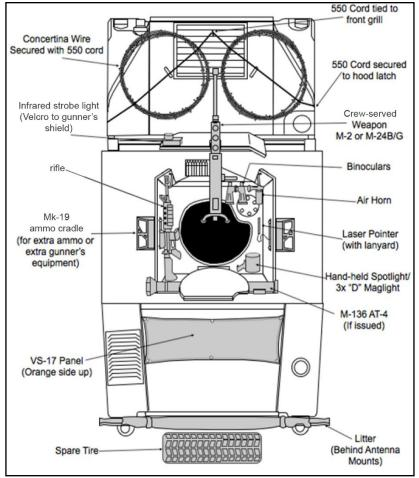
Figure 7-2. Example HMMWV Exterior Packing and Load Plan.
