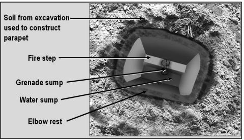
Figure 4-6. Step 3 of Fighting Position Preparation (overhead view).
