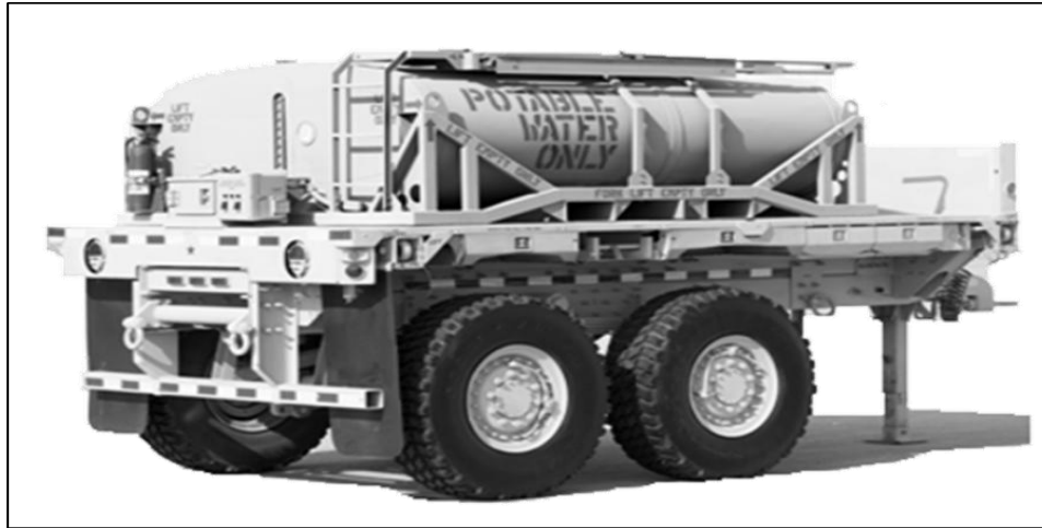
Figure A-15. Unit water pod system (Camel II)
