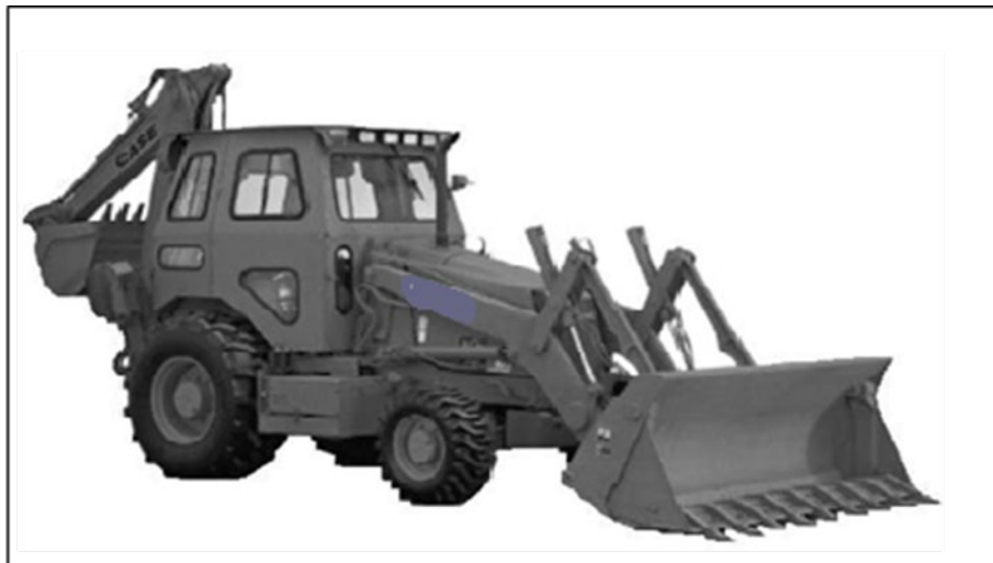
Figure 8-1. Backhoe loader (BHL)
