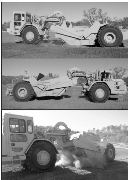
Figure 3-2. Functions of the apron, bowl, and ejector
