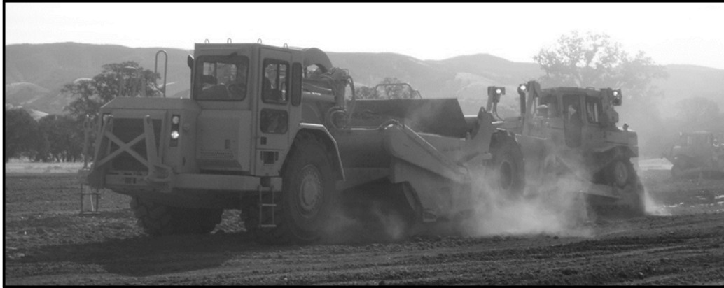
Figure 3-3. Straddle loading with pusher assistance
