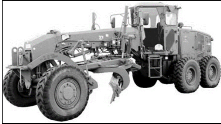
Figure B-4. 120M motorized road grader
