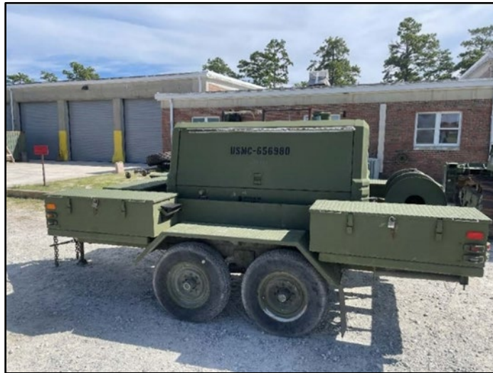
Figure 9-1. Trailer-mounted, 260-cfm air compressor
