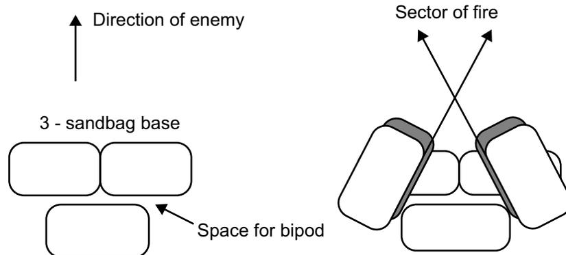
**Figure 2-22. Sandbag Sector Method of Field Expedient Lay.**
