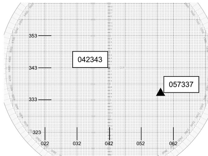
**Figure 3-36. Marking the Y Coordinates and Observer Position—Board Setup Complete.**
