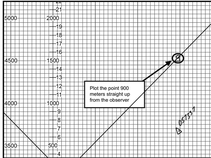
Figure 3-50. Plotting New Target—Direction 0820, Distance 900.
