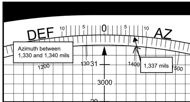
Figure 3-39. Reading the Azimuth from the Vernier Scale.
