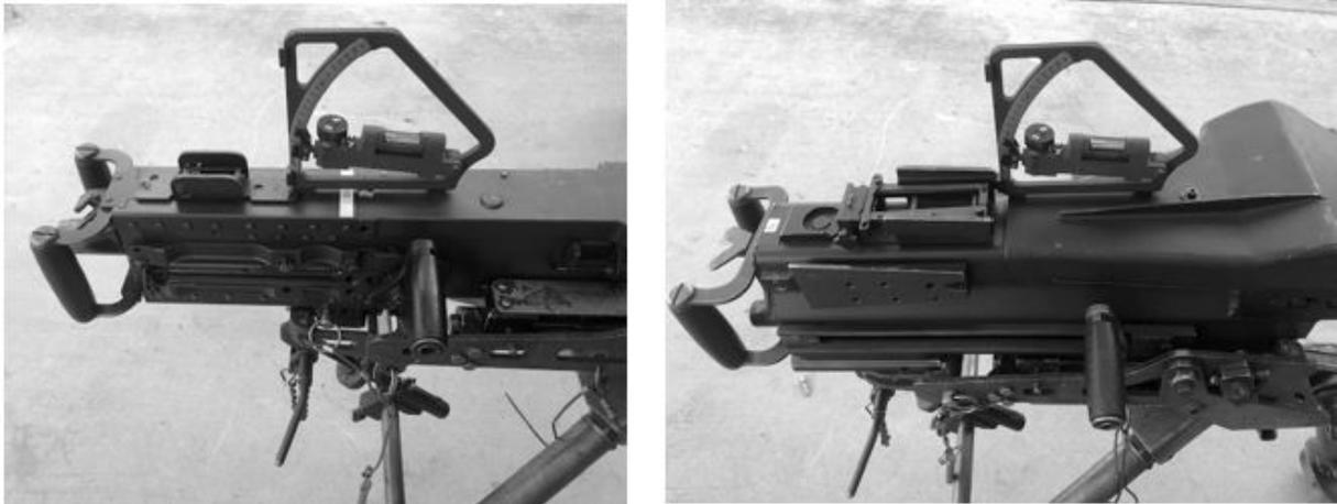
**Figure 3-9. Setting Quadrant Elevation on a Gun with the M2A1.**
