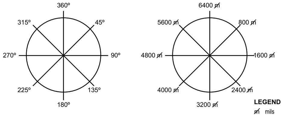
Figure 2-2. Illustration of Degrees and Mils.
