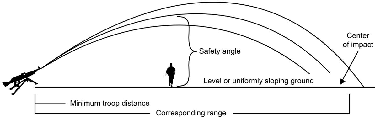
**Figure 3-19. Corresponding Range and Minimum Troop Distance.**
