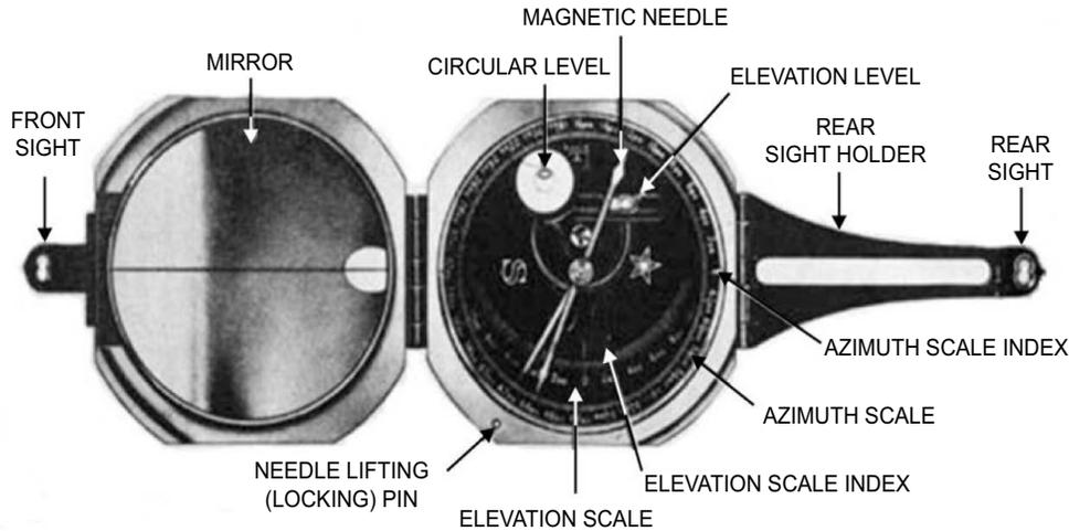
**Figure 3-11. M2 Compass and Components.**
