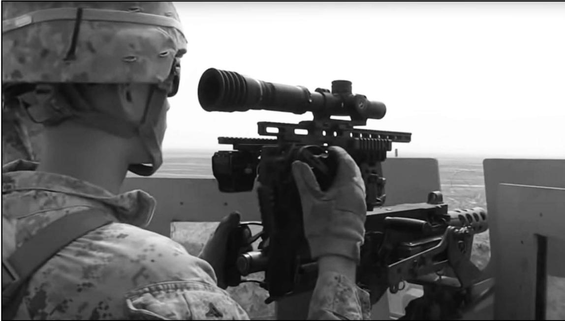
Figure 4-8. Vehicle-Mounted M2A1 Heavy Machine Gun with Heavy Machine Gun Sight System.
