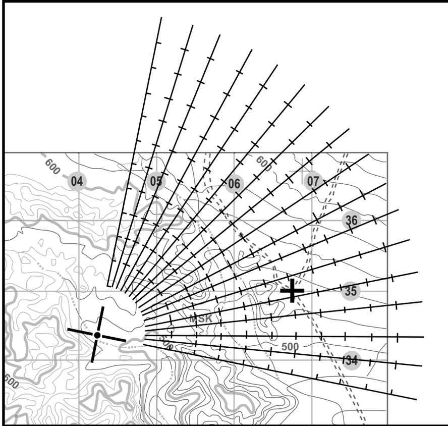
Figure 3-61. Using the Observed Fire Fan with a Map.
