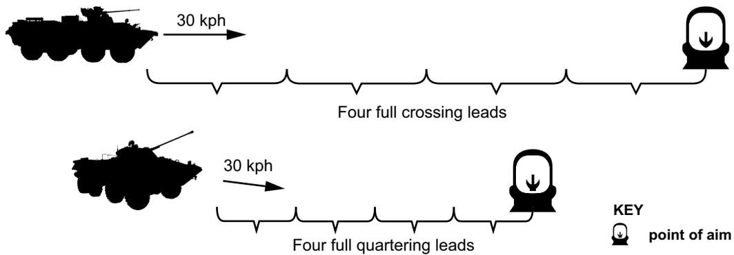
**Figure 3-70. Crossing Leads and Quartering Leads for a Vehicle Moving 30 kph, 900 Meters from the Gun.**
