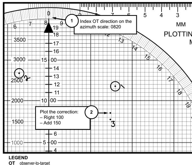
**Figure 3-53. Plotting the Correction.**
