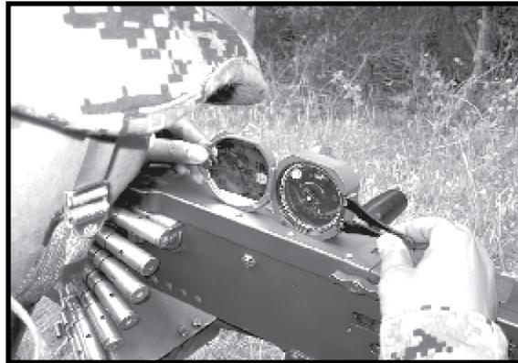
**Figure 3-12. Setting Quadrant Elevation with the M2 Compass.**
