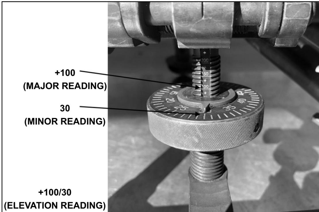
Figure 2-17. Traversing and Elevating Mechanism Readings (Example 2).
