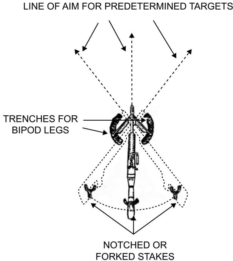
Figure 2-21. Forked Stake Method.
