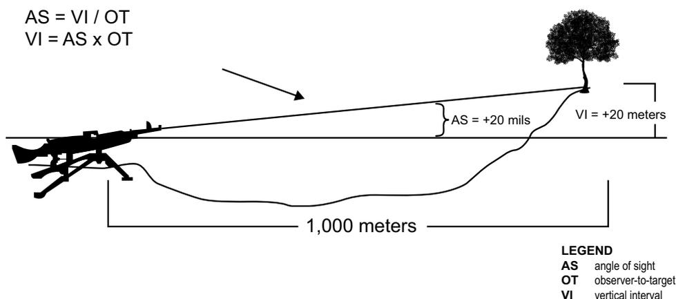
Figure 3-3. Vertical Interval.
