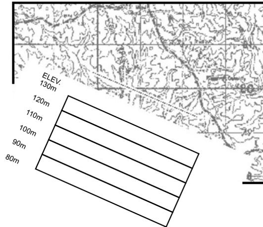
**Figure 3-63. Horizontal Lines and Corresponding Elevations.**
