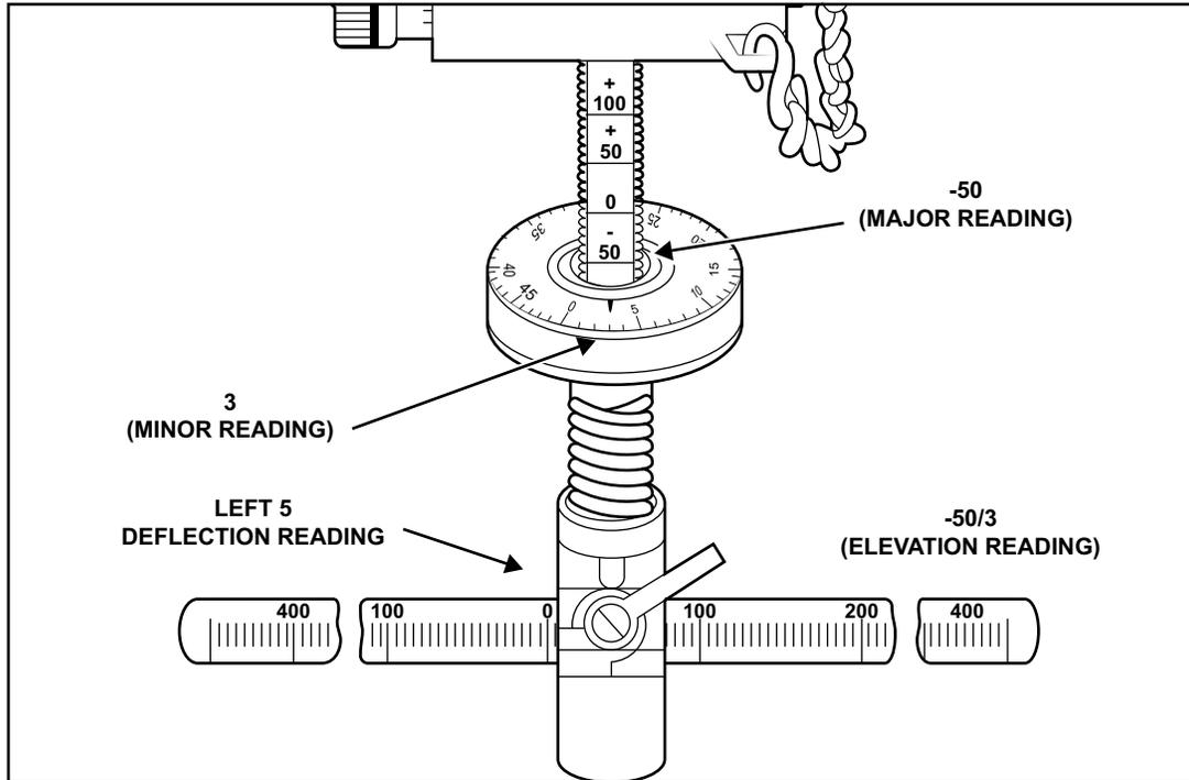
Figure 2-16. Traversing and Elevating Mechanism Readings (Example 1).
