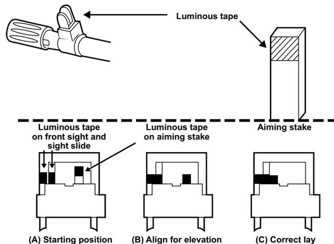
**Figure 2-20. Luminous Aiming Stake Method of Field Expedient Lay.**
