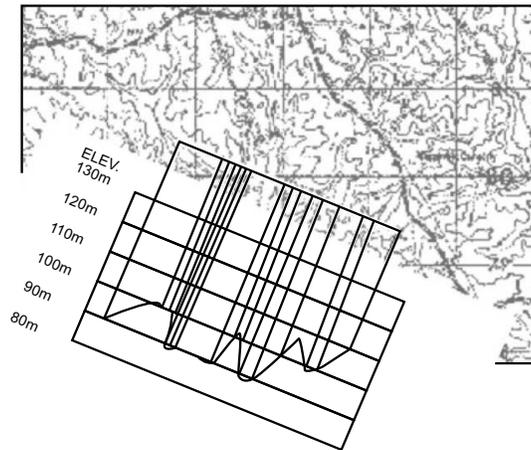
**Figure 3-65. Connect the Contour Points with a Smooth Curve.**
