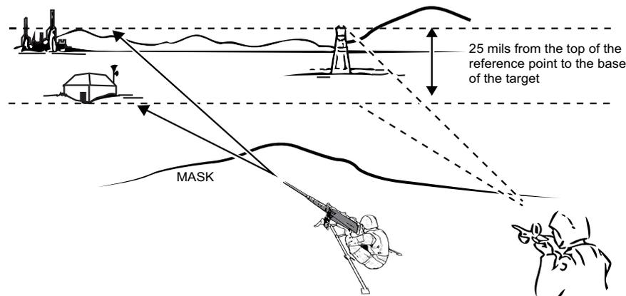
**Figure 3-25. Laying a Gun for Elevation by Reference Point.**
