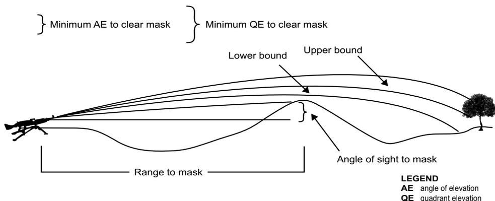
**Figure 3-26. Cone of Fire Clearing the Mask.**
