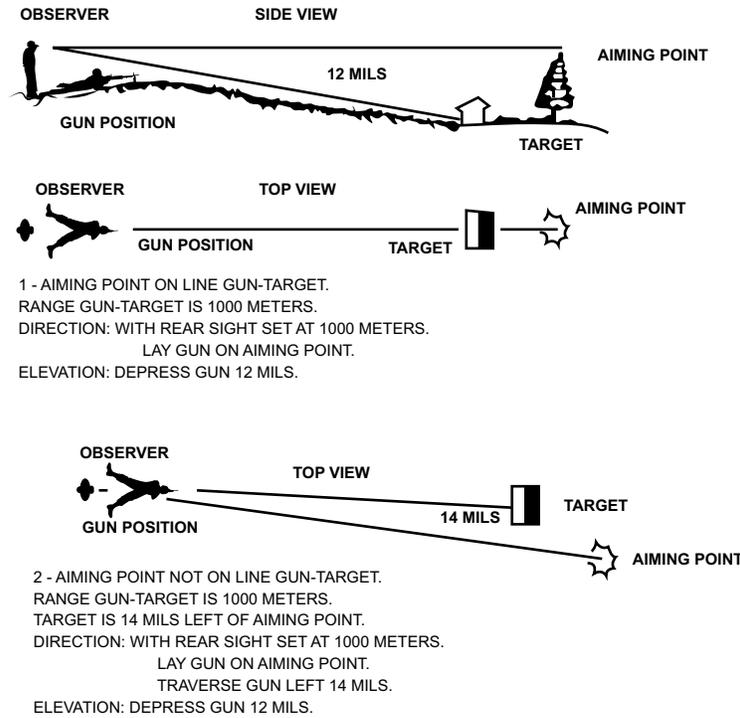
Figure 2-23. Aiming Point Method.
