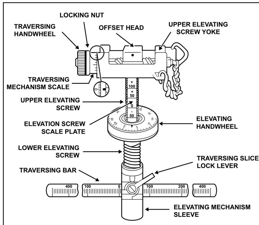
Figure 2-12. Traversing and Elevating Mechanism for the M240B.
