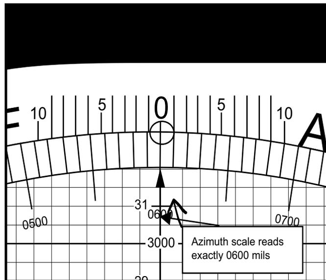
Figure 3-43. Reading Azimuth of 0600 Vernier Scale.
