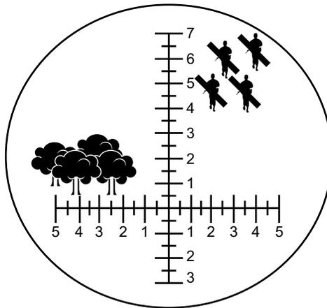
**Figure 3-18. Determining Overhead Safety Limit with Binoculars.**
