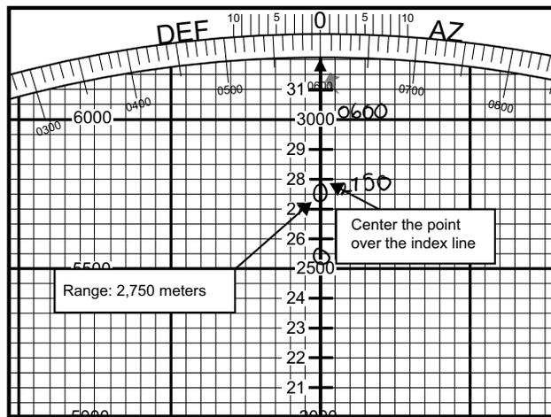
Figure 3-46. Indexing the Correction.
