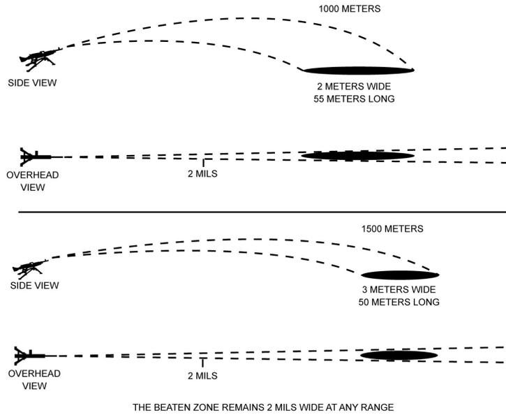
Figure 1-6. Effect of Range on the Beaten Zone (Example Shown for M240B).
