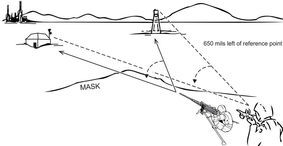
**Figure 3-22. Laying the Gun for Direction by Reference Point.**
