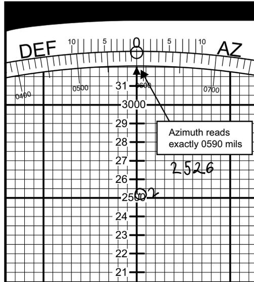
Figure 3-47. Reading an Azimuth of 0590 with the Vernier Scale.
