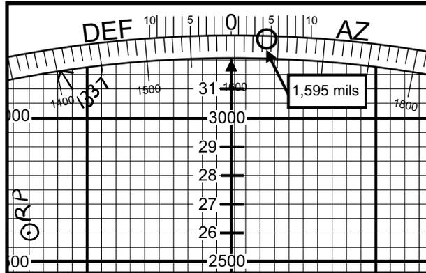
Figure 3-52. Reading an Azimuth of 1,595 with the Vernier Scale.
