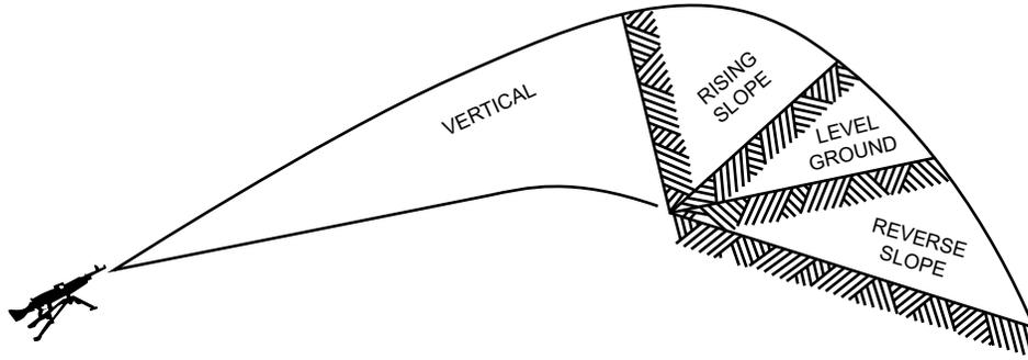
Figure 1-5. Effect of Ground Slopes on the Beaten Zone.
