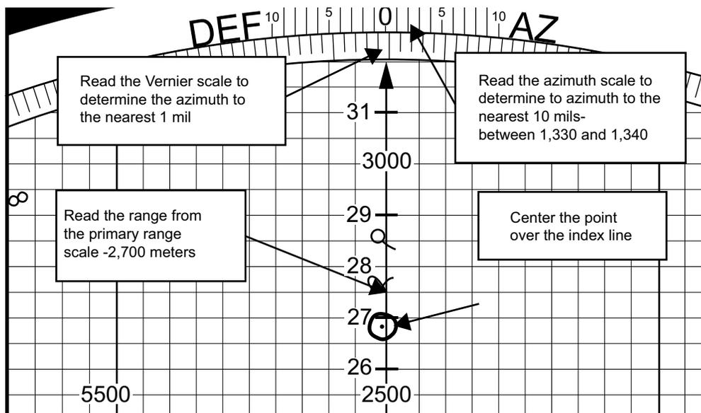
Figure 3-38. Indexing the Point to Determine Azimuth and Range.
