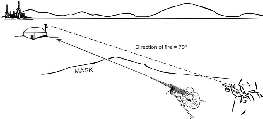
Figure 3-24. Laying the Gun on the Direction Obtained from the Map.
