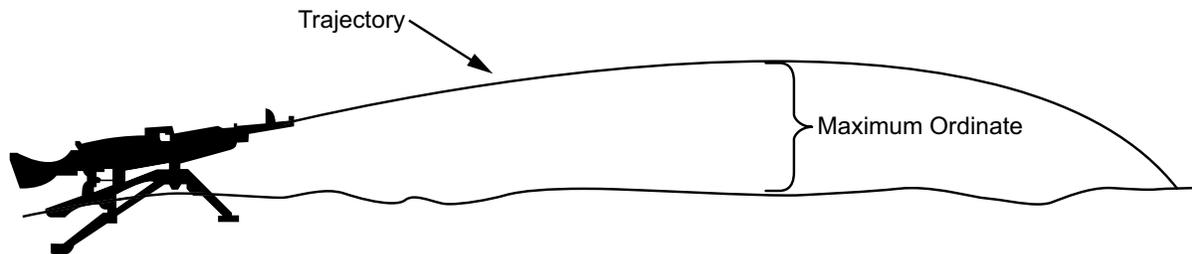
Figure 1-1. Trajectory and Maximum Ordinate.
