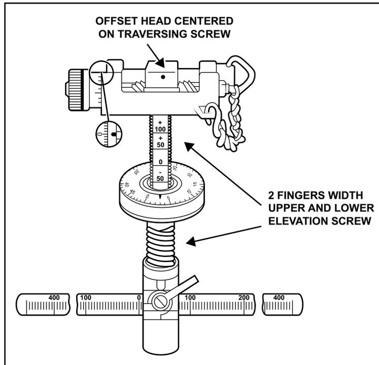
Figure 2-14. Zeroed Traversing and Elevating Mechanism.
