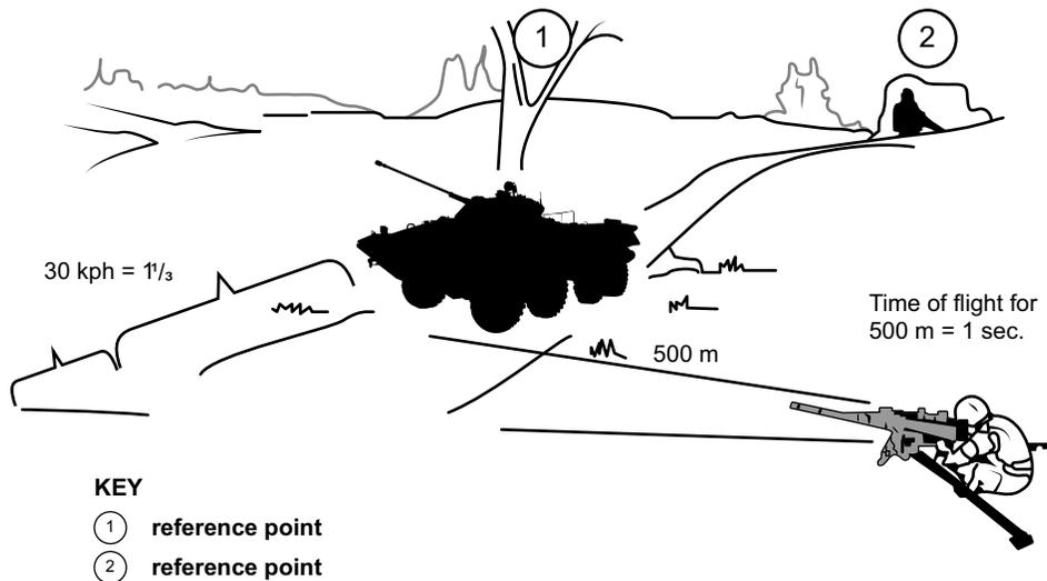
**Figure 3-71. Estimating the Speed of a Moving Vehicle.**
