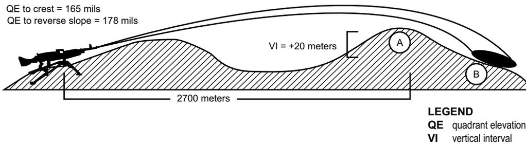
**Figure 3-68. Calculating Quadrant Elevation to Search a Reverse Slope.**
