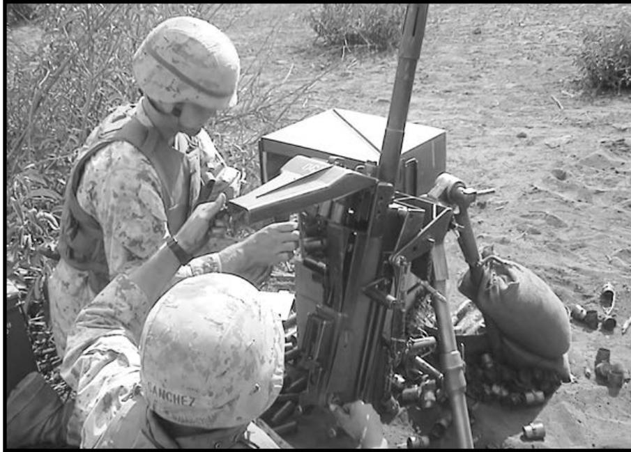
**Figure 3-20. MK-19 Set Up for High-Angle Fire.**
