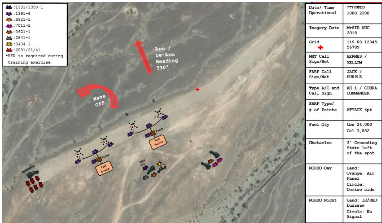
Figure D-3. Notional Attack (HOT) Forward Arming and Refueling Point Diagram.
