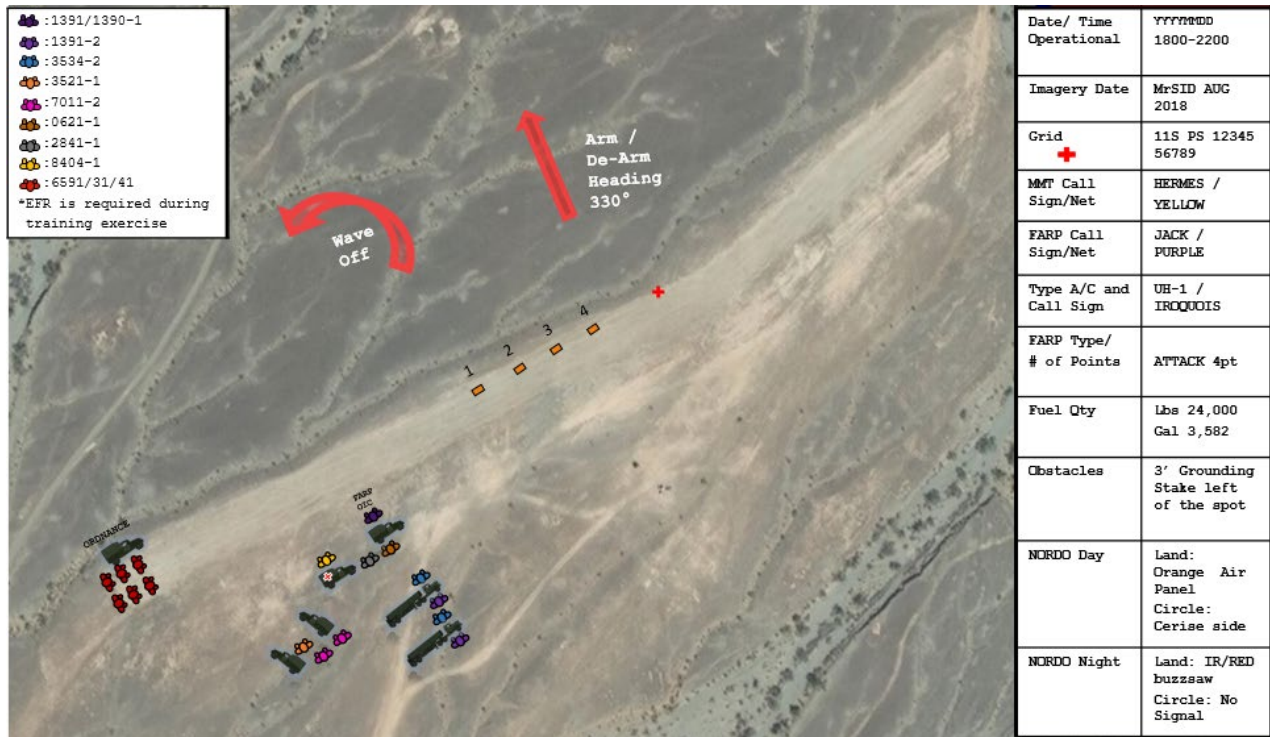
Figure D-4. Notional Attack (COLD) Forward Arming and Refueling Point Diagram.
