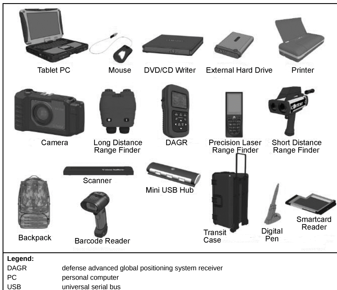
Figure E-1. ENFIRE components
