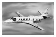
The UC-35 is a medium range executive and priority cargo jet aircraft. It is a commercial off the shelf version of the military Cessna Citation 560 Ultra V UC-35C or Encore UC-35D twin-engine aircraft. The military version includes a wider cargo door, mode I-IV IFF, AN/ARC 210 satellite communications with embedded encryption (KY-58 capable) and DAMA modem radio, high frequency radio, and flight phone.
