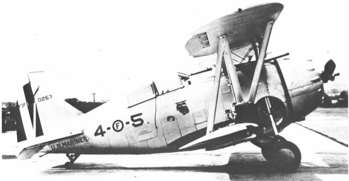
*An F3F-1 of VF-4M. This was the first Marine fighter with retractable landing gear. (Photo from Museums Branch Activities, Quantico).*
