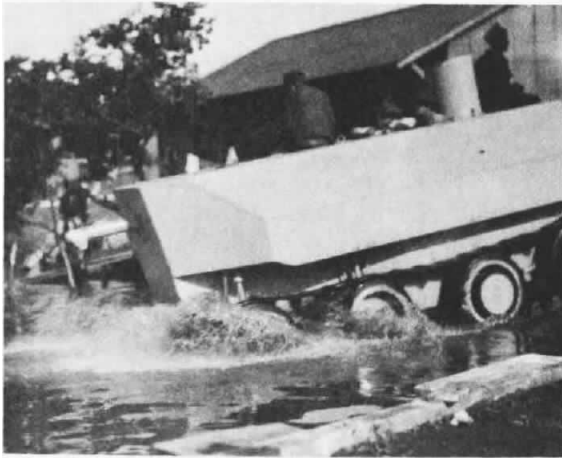
Christie amphibian tank, mounting a 75mm gun, is tested at the Culebra maneuvers in 1924. (USMC Photo #523115).
