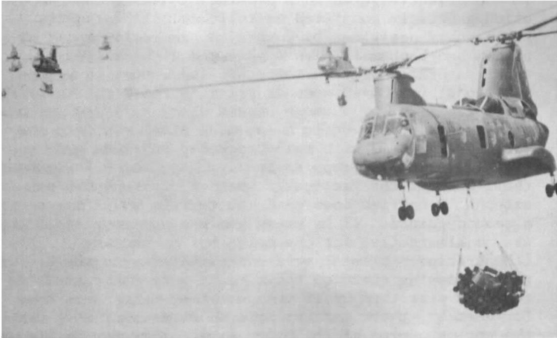
After introduction of the Super Gaggle, CH-46 helicopters with their 4,000-pound external loads proceeded to the hill outposts in convoy. (USMC Photo A422061)
