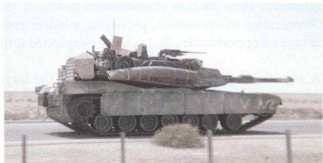
*To extend the Division's logistical culminating point, vehicles were fitted with external fuel reserves, such as these FLEXCELL fuel bladders on an M1A1.*
