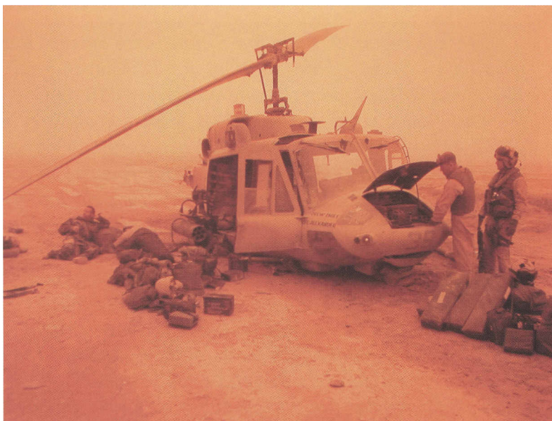
The sandstorm took its toll on machines as well as aircraft. This UH-1N crashed because of dirt and debris blown into the engine.
