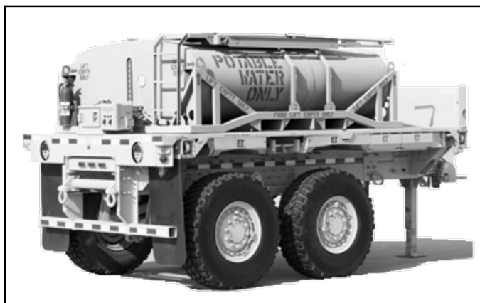
Figure 5-6. Unit Water Pod System (Camel II)
