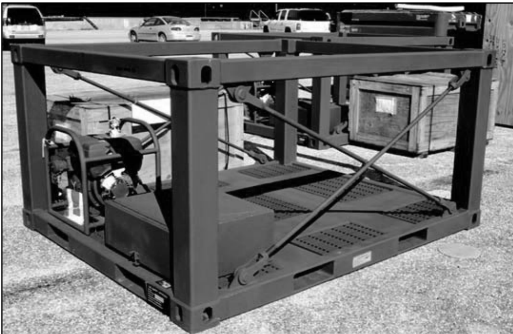
Figure 5-9. Six Container (SIXCON) Water Pump Module
