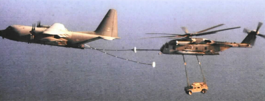
Photo by: Cpl Paula M. Fitzgerald A CH-53E Super Stallion helicopter prepares to receive fuel from a KC-130 Hercules aircraft during an aerial refueling exercise. The helicopter belonged to Marine Heavy Helicopter Squadron 772, a reserve squadron from Willow Grove, Pennsylvania, that served with the 24th Marine Expeditionary Unit (Special Operations Capable) in support of Operation Enduring Freedom.
