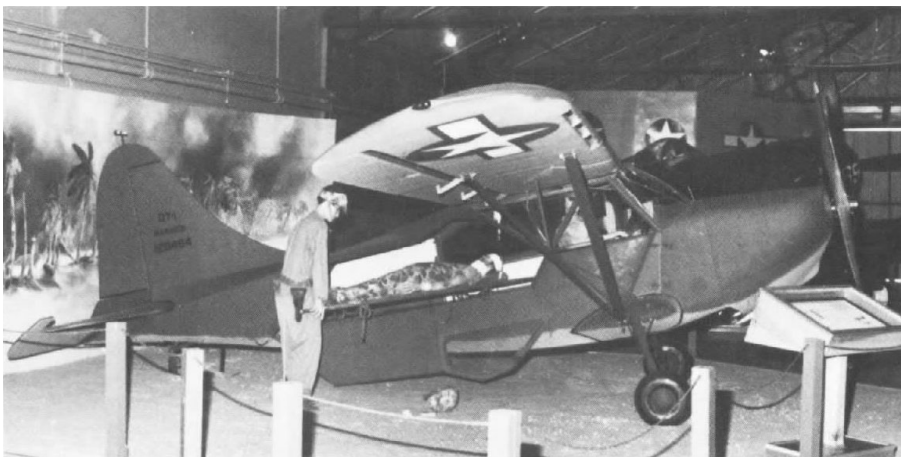
In addition to its use as an artillery spotting platform, the OY-2 Sentinel was also valuable to Marine combat troops for the medical evacuation capabilities it provided.
