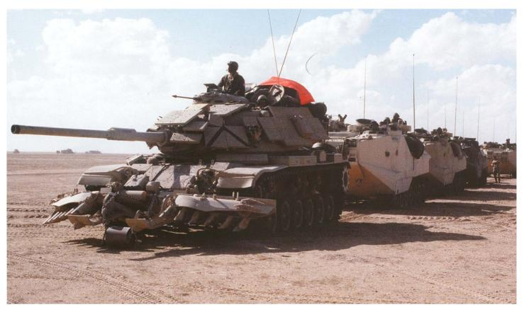
M-60A1 main battle tank equipped with reactive armor, mine-clearing rollers and plow stand by at the head of a column of AAVP-7A1 assault amphibian vehicles as I MEF prepares to enter Kuwait at the start of the ground phase of Operation "Desert Storm".
