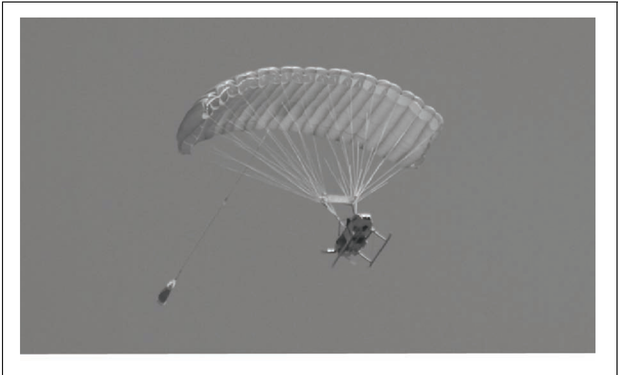
Figure 6-1. The Wind Supported Aerial Delivery System (Snow Goose)
