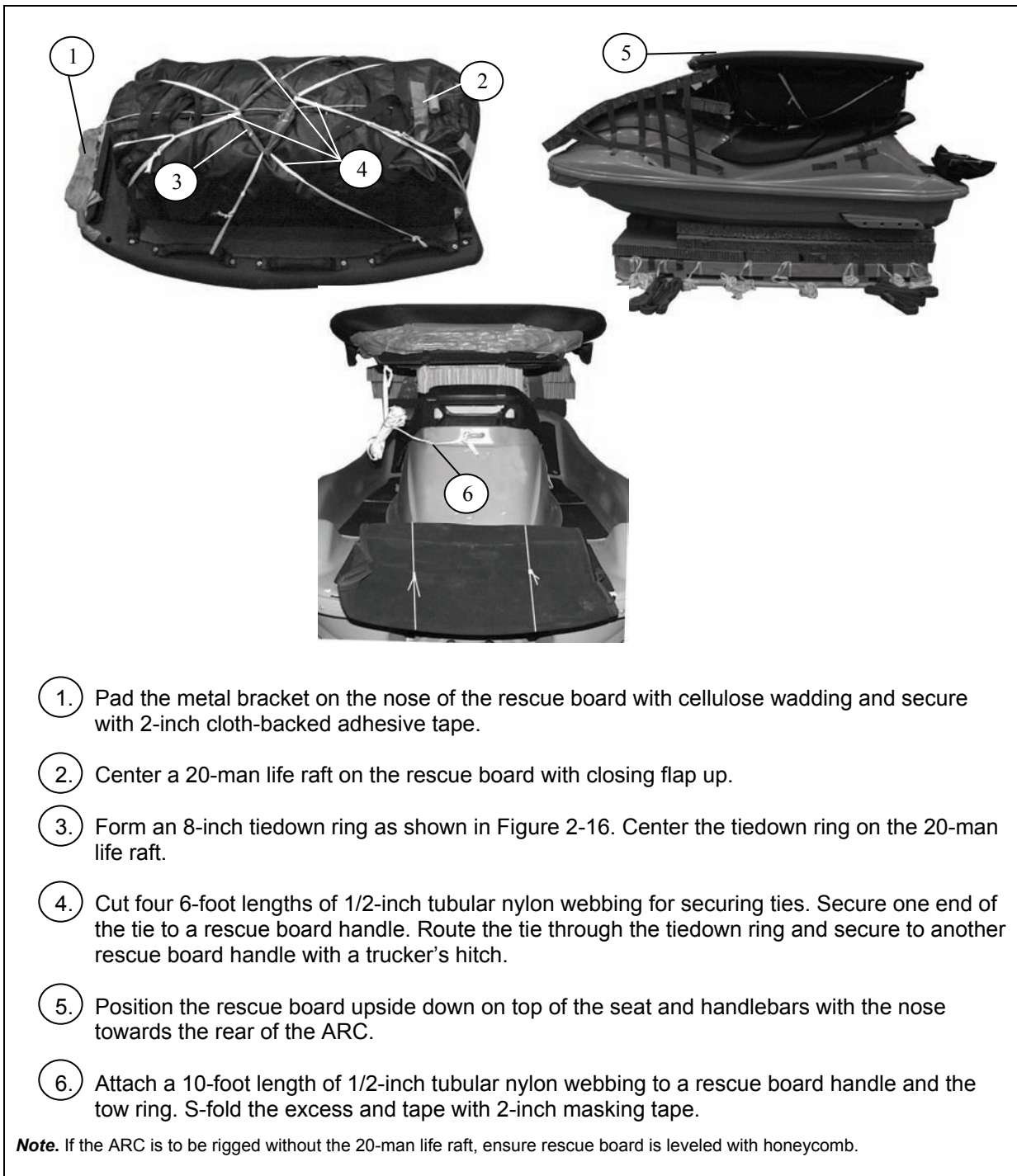
Figure 5-22. Rescue Board Installed
