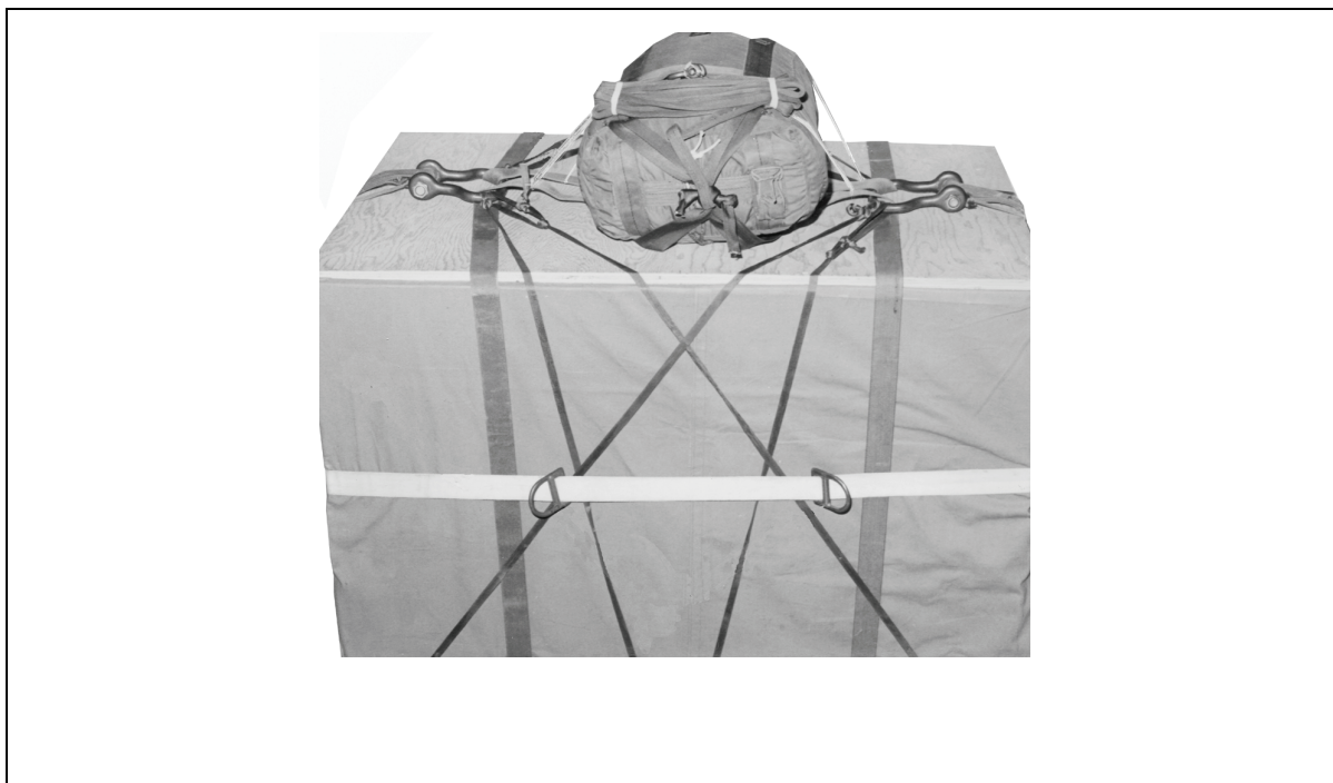
Figure 1-1. High Speed Low Level Aerial Delivery System (HSSLADS)
