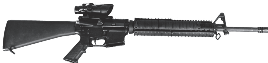
Figure 3-11. Rifle Combat Optic Mounted on M16A4.
