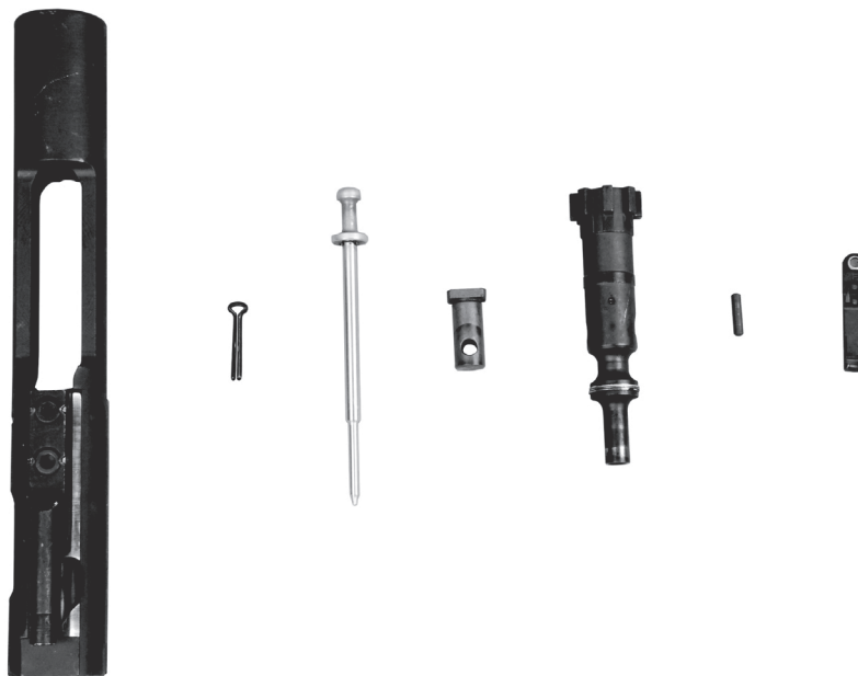
Figure 3-35. Bolt Carrier Disassembled.
