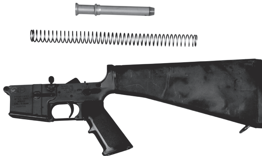
Figure 3-36. Lower Receiver Disassembled.
