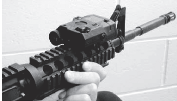
Figure 15-4. Top Mount on M4/M4A1.
