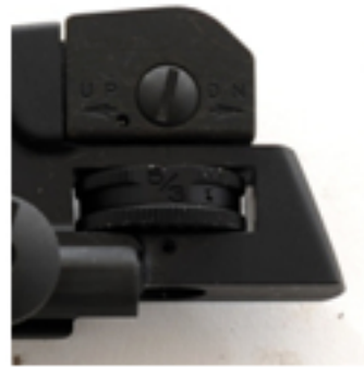
Figure 8-18. Elevation Knob Set at 6/3.
