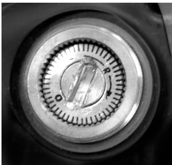
Figure 8-3. Service Rifle Combat Optic Windage Adjuster.
