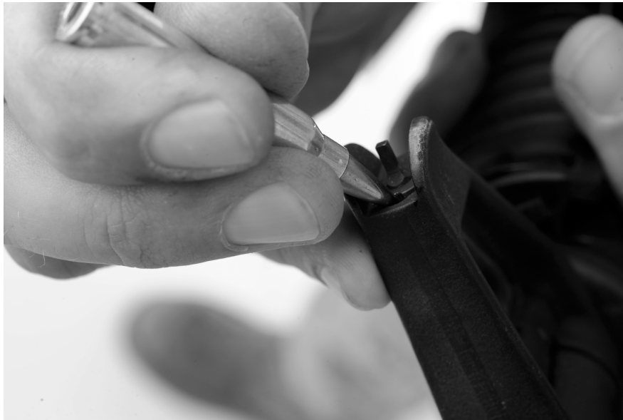
Figure 8-12. Front Sight Adjustment.
