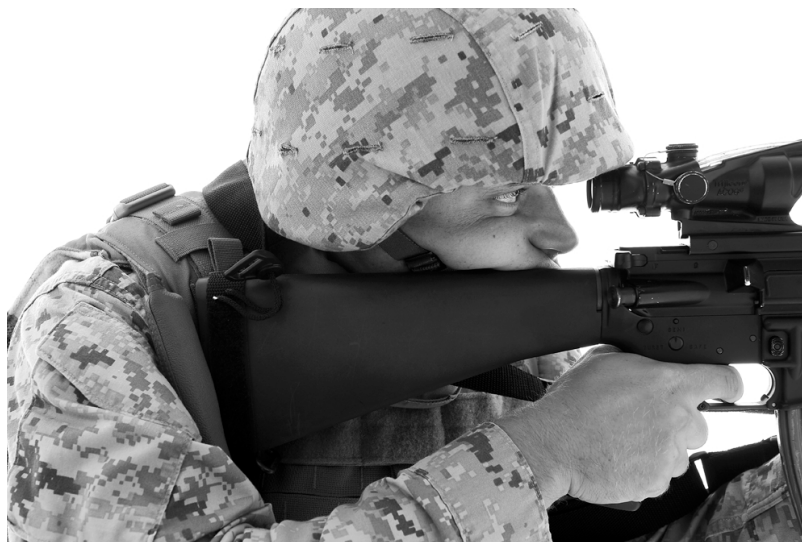
Figure 5-4. Proper Eye Relief with the Rifle Combat Optic.
