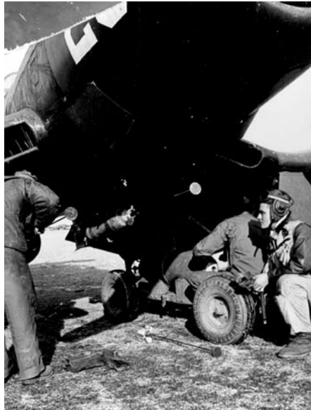
Department of Defense Photo (USMC) A130488 Marines who used the "daisy-cutter" in the South Pacific rig them again for use against the Chinese in Korea. Attaching the bombs to the racks of the Corsair required delicate adjustments, often difficult in the sub-zero Korean winter weather.
