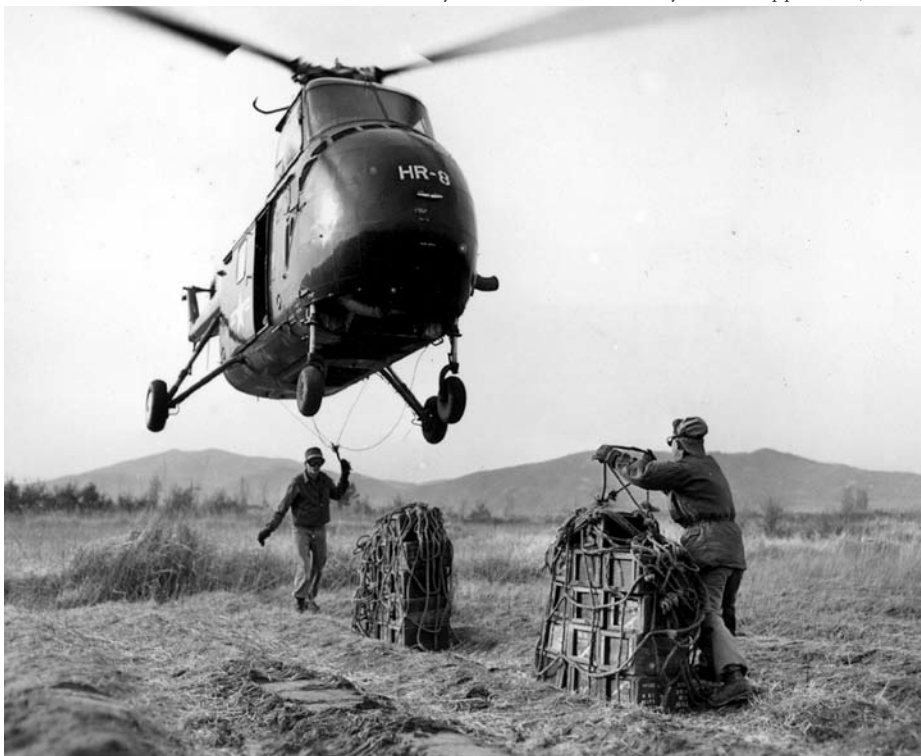
A helicopter from HMR-161 prepares to lift bundled supplies from the 1st Air Delivery Platoon area to frontline troops. The air delivery platoon signalman holds the hook while the other Marine holds the net in a hook-up position.
